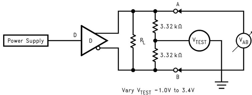
**Figure 3. Differential Driver Full Load Test Circuit**
