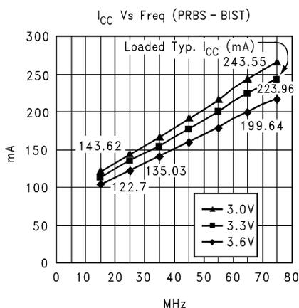
Figure 10.  $I_{CC}$  vs Freq
