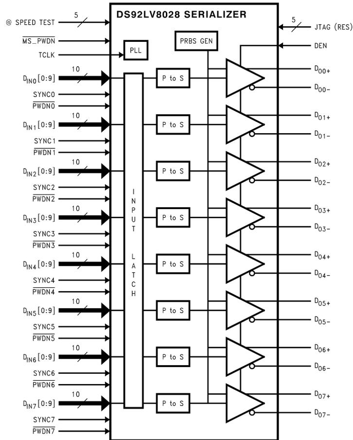
Figure 11. DS92LV8028 Functional Block Diagram
