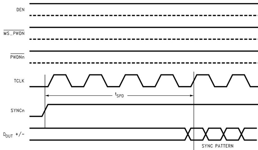
Figure 8. SYNC Timing Delays
