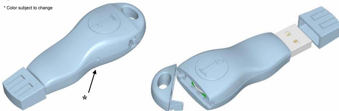
**\*Note:** To eject an iButton, insert a straightened paper clip into the side access hole of the DS9490B. Push the paper clip in the direction of the iButton. A different iButton can then be inserted. The data contact faces down and away from the embossed ‘i’. Before inserting the paper clip disconnect the DS9490B from the USB bus.
