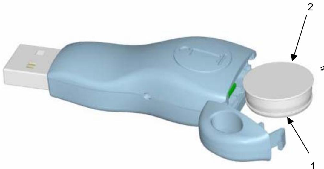
**\*Note:** The data contact faces down and away from the embossed ‘i’. Once the iButton is inserted in the enclosure, snap the end cap over it. The end cap is removed by depressing the release tab, swinging it fully open, and sliding out the hinge.
