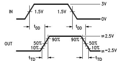
(1) The input pulse is supplied by a generator having the following characteristics: PRR = 1.0 MHz, duty cycle ≈ 50%,  $t_r \leq 6.0$  ns,  $t_f \leq 6.0$  ns,  $Z_O = 50\Omega$ .
