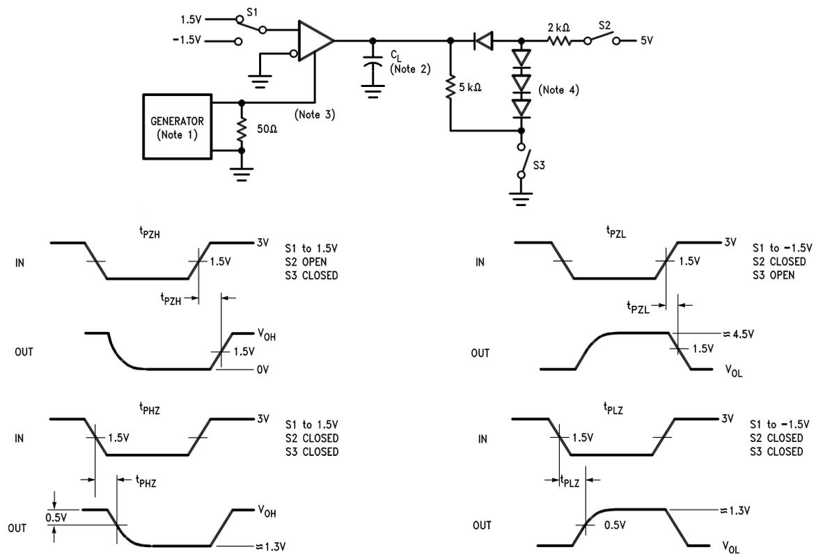
(1) The input pulse is supplied by a generator having the following characteristics: PRR = 1.0 MHz, duty cycle  $\approx$  50%,  $t_r \leq 6.0$  ns,  $t_f \leq 6.0$  ns,  $Z_O = 50\Omega$ .
