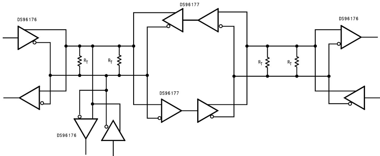
The line length should be terminated at both ends in its characteristic impedance.
