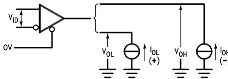
Figure 4. Receiver  $V_{OH}$  and  $V_{OL}$
