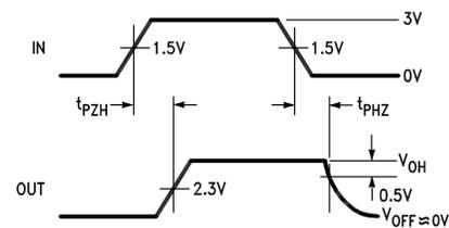
(1) The input pulse is supplied by a generator having the following characteristics: PRR = 1.0 MHz, duty cycle ≈ 50%,  $t_r \leq 6.0$  ns,  $t_f \leq 6.0$  ns,  $Z_O = 50\Omega$ .
