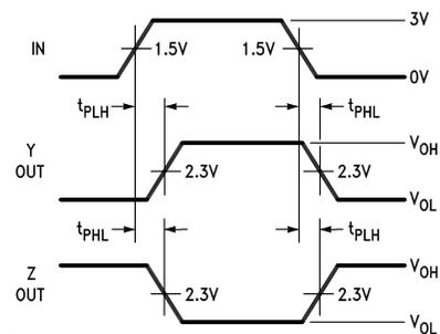
(1) The input pulse is supplied by a generator having the following characteristics: PRR = 1.0 MHz, duty cycle ≈ 50%,  $t_r \leq 6.0$  ns,  $t_f \leq 6.0$  ns,  $Z_O = 50\Omega$ .
