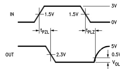
(1) The input pulse is supplied by a generator having the following characteristics: PRR = 1.0 MHz, duty cycle ≈ 50%,  $t_r \leq 6.0$  ns,  $t_f \leq 6.0$  ns,  $Z_O = 50\Omega$ .
