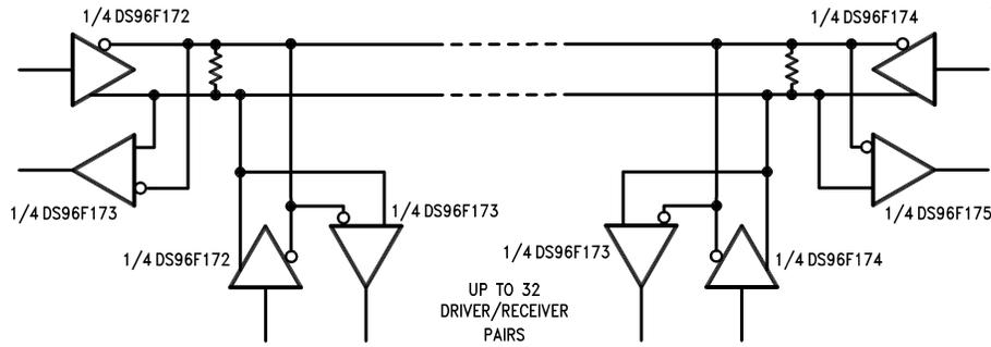
The line length should be terminated at both ends in its characteristic impedance.
