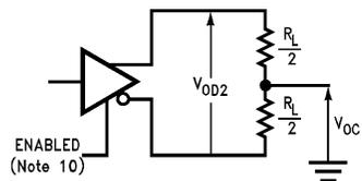
**Note 10:** DS96F172 with active high and active low Enables is shown. DS96F174 has active high Enable only.
