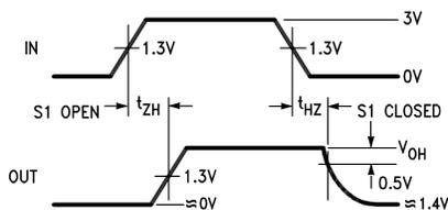
Figure 8.  $t_{HZ}$ ,  $t_{ZH}$
