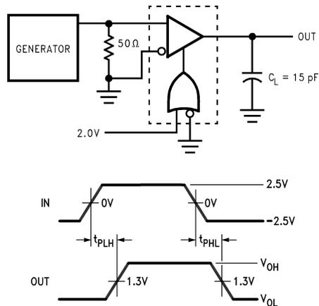
Figure 7.  $t_{PLH}$ ,  $t_{PHL}$
