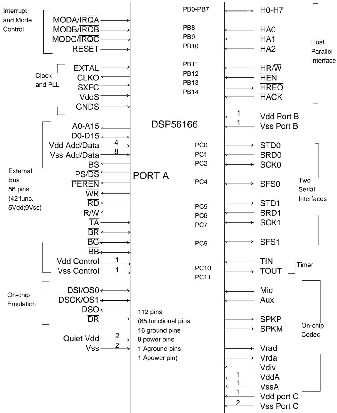
**Figure 3 DSP56166 Pinout**
