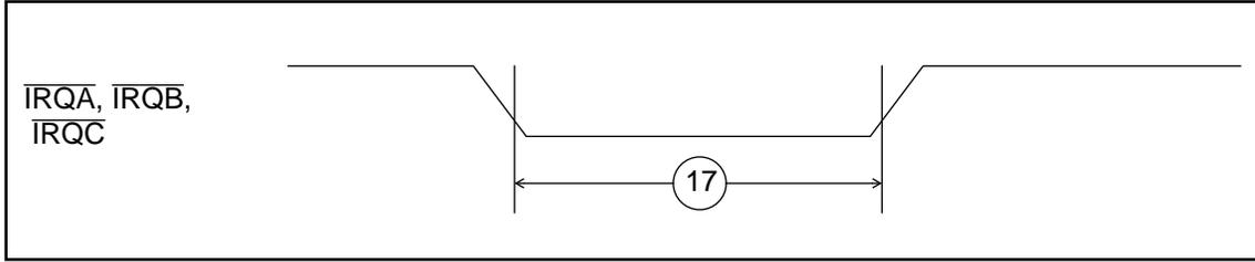
**Interrupt Figure 4. External Interrupt Timing (Negative Edge-Triggered)**
