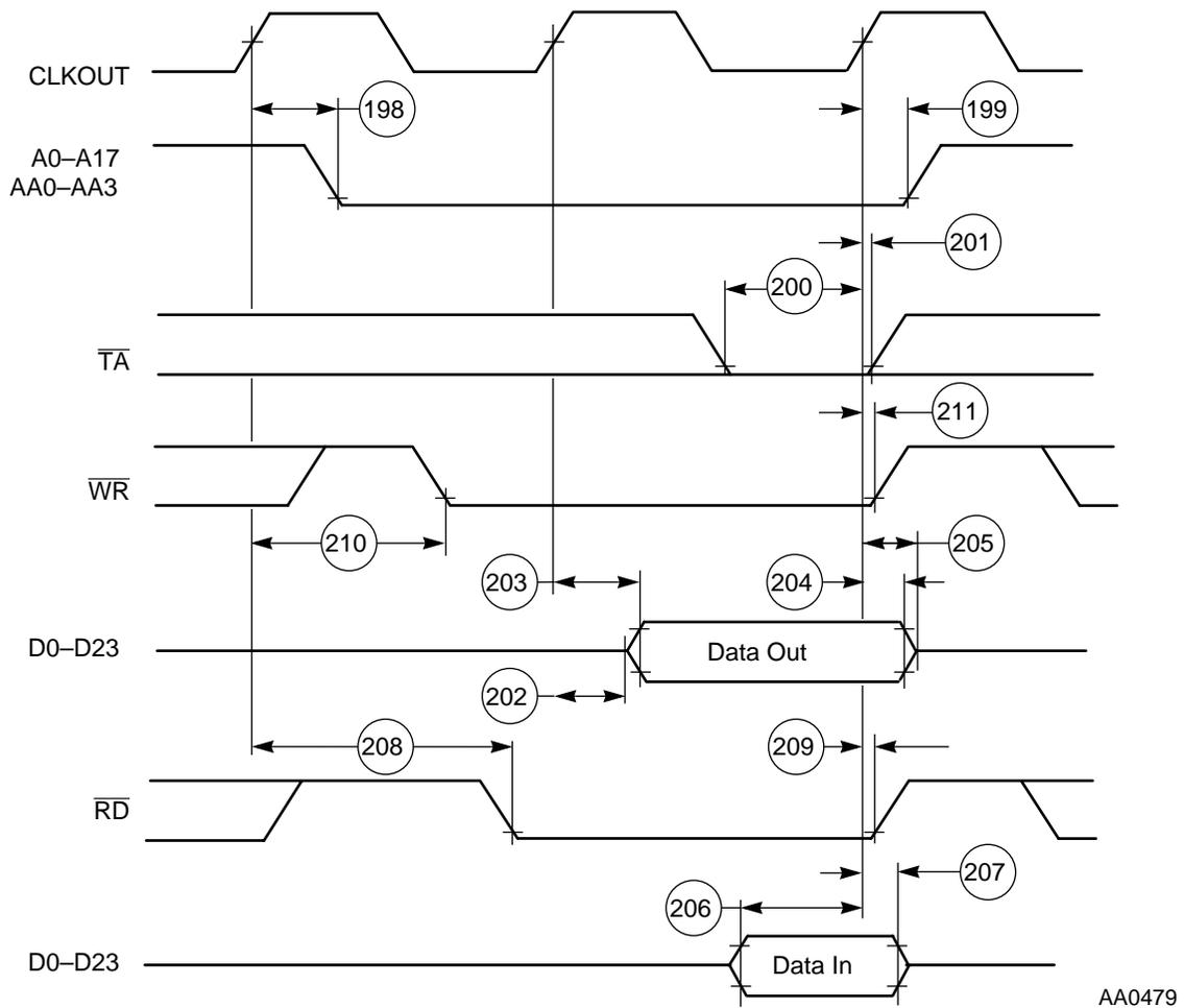
Figure 2-21 Synchronous Bus Timings 1 WS (BCR Controlled)
