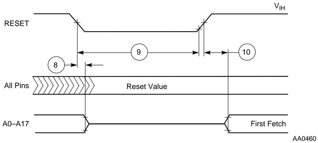
Figure 2-3 Reset Timing
