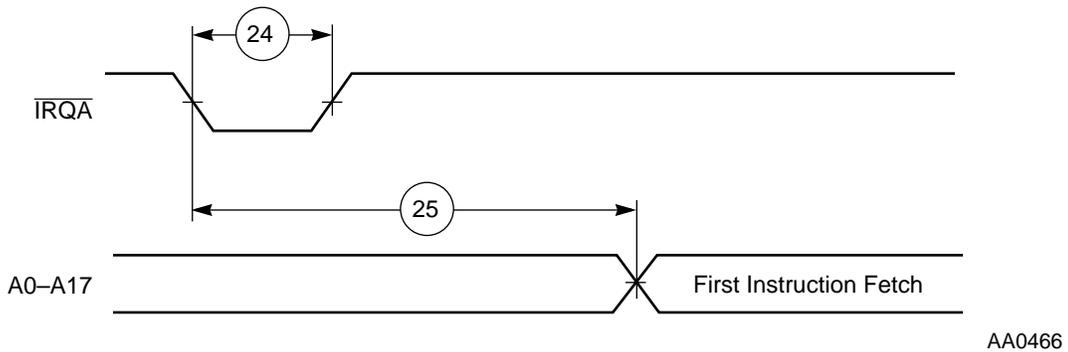
Figure 2-9 Recovery from Stop State Using  $\overline{IRQA}$
