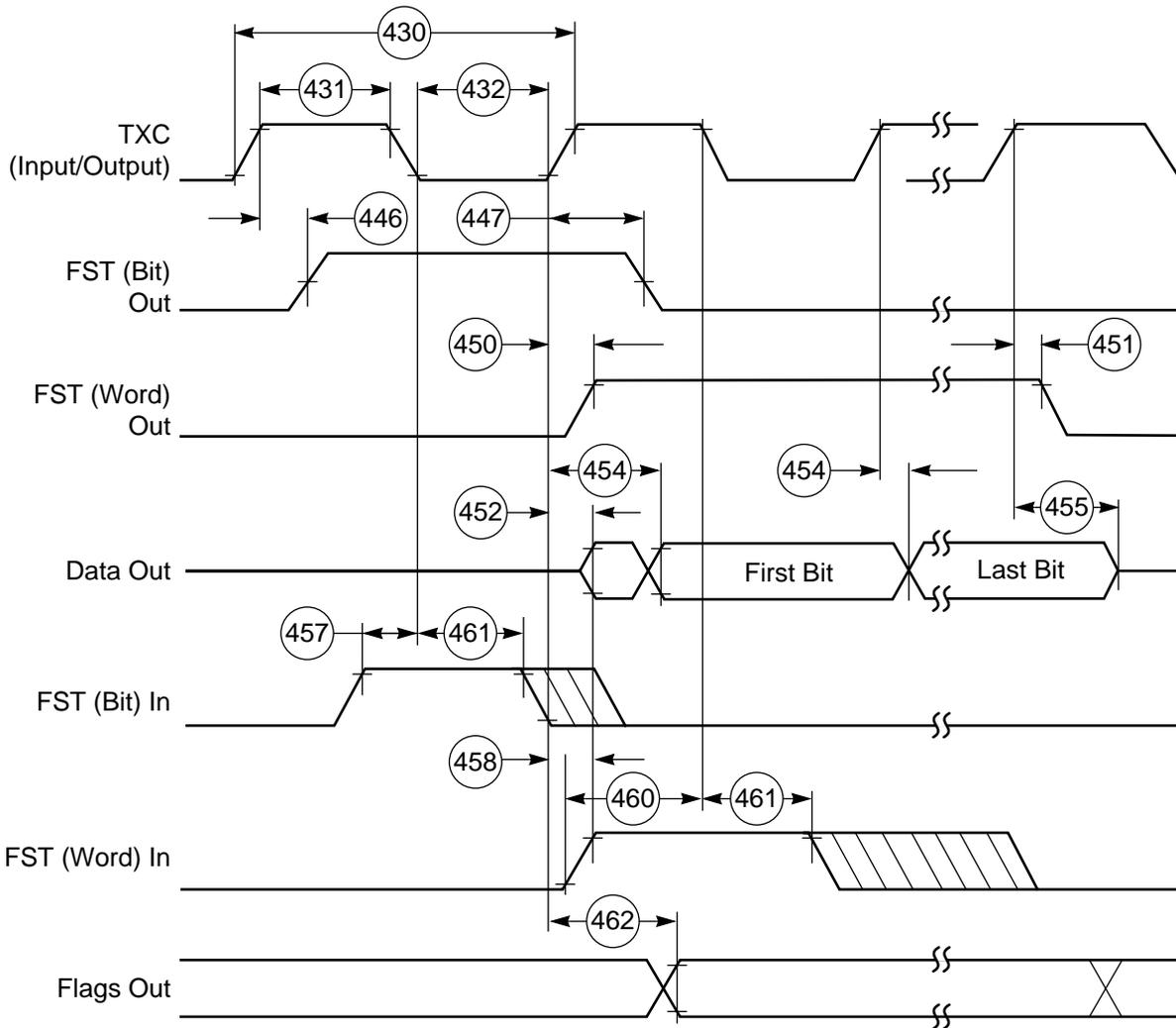
Note: In Network mode, output flag transitions can occur at the start of each time slot within the frame. In Normal mode, the output flag state is asserted for the entire frame period.
