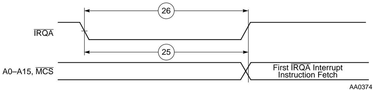
Figure 2-10 Recovery from Stop Using  $\overline{IRQA}$  Interrupt Service
