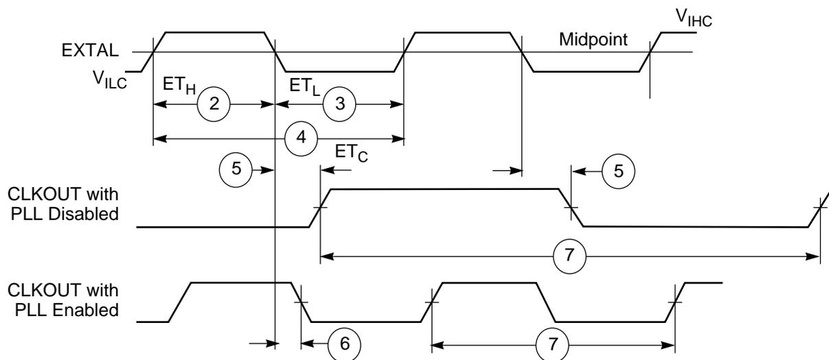
Note: The midpoint is  $0.5(V_{IHC} + V_{ILC})$ .
