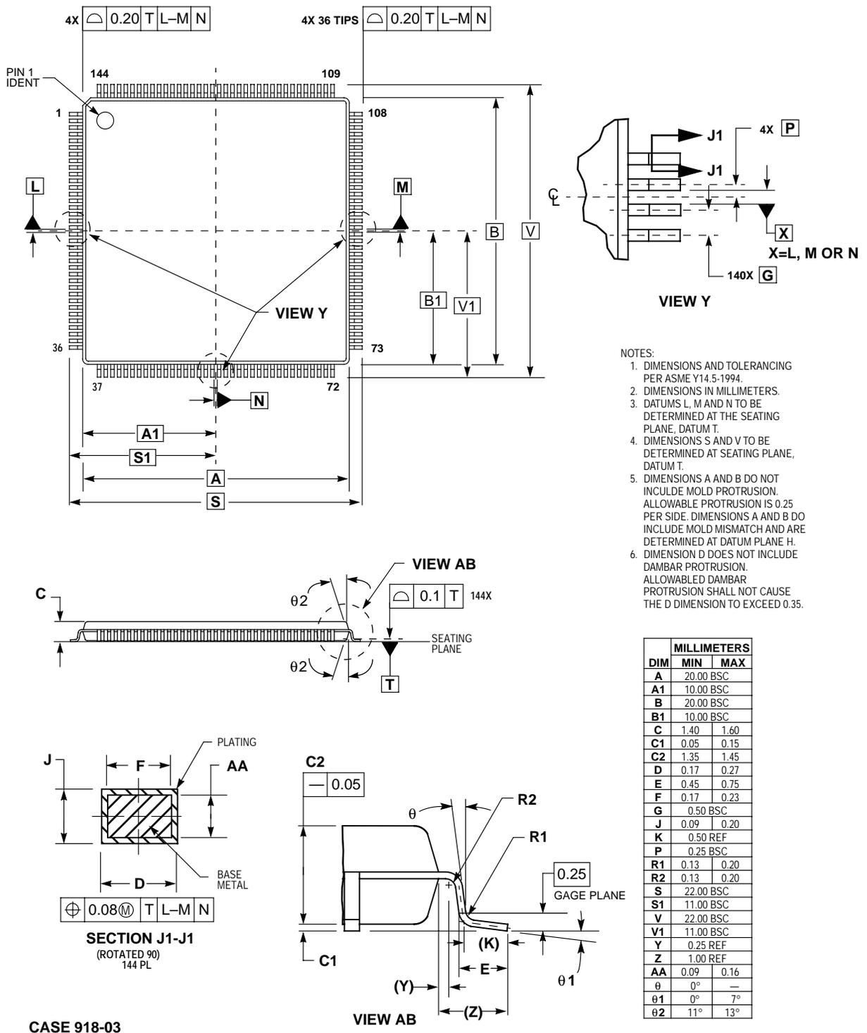
Figure 3-3 144-pin Thin Quad Flat Pack (TQFP) Mechanical Information
