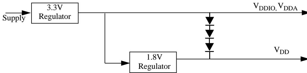
**Figure 4. Example Circuit to Control Supply Sequencing**
