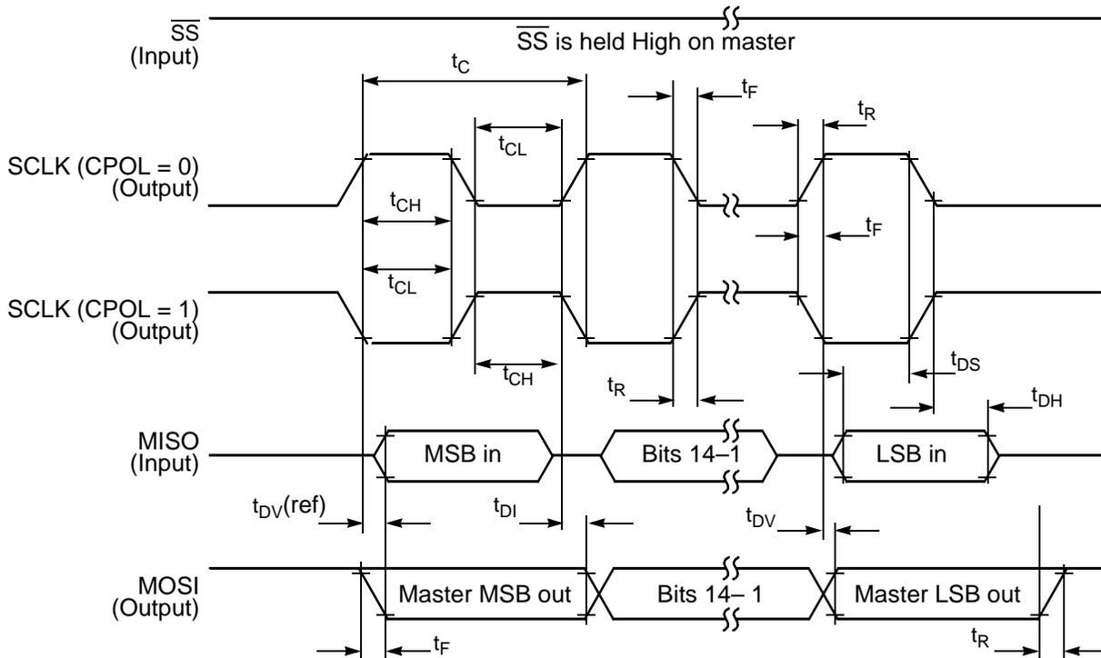
Figure 25. SPI Master Timing (CPHA = 1)
