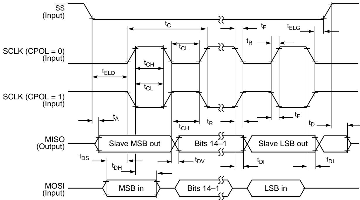
**Figure 26. SPI Slave Timing (CPHA = 0)**
