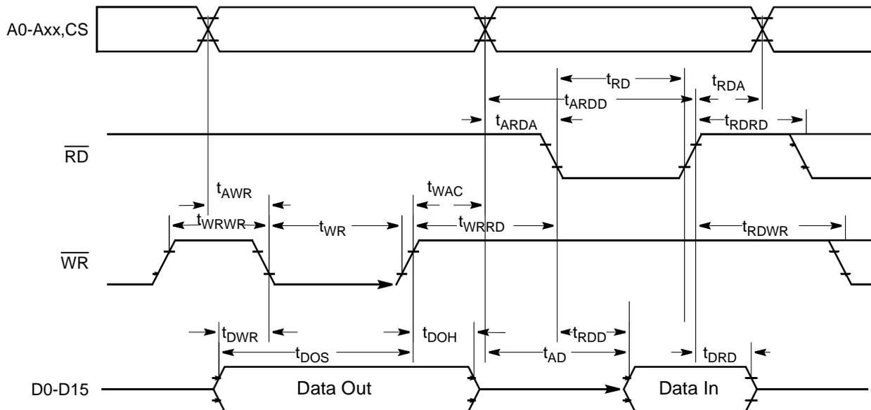
Note: During read-modify-write instructions and internal instructions, the address lines do not change state.
