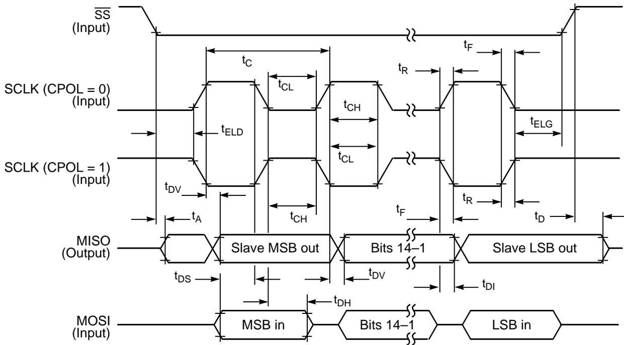
**Figure 27. SPI Slave Timing (CPHA = 1)**
