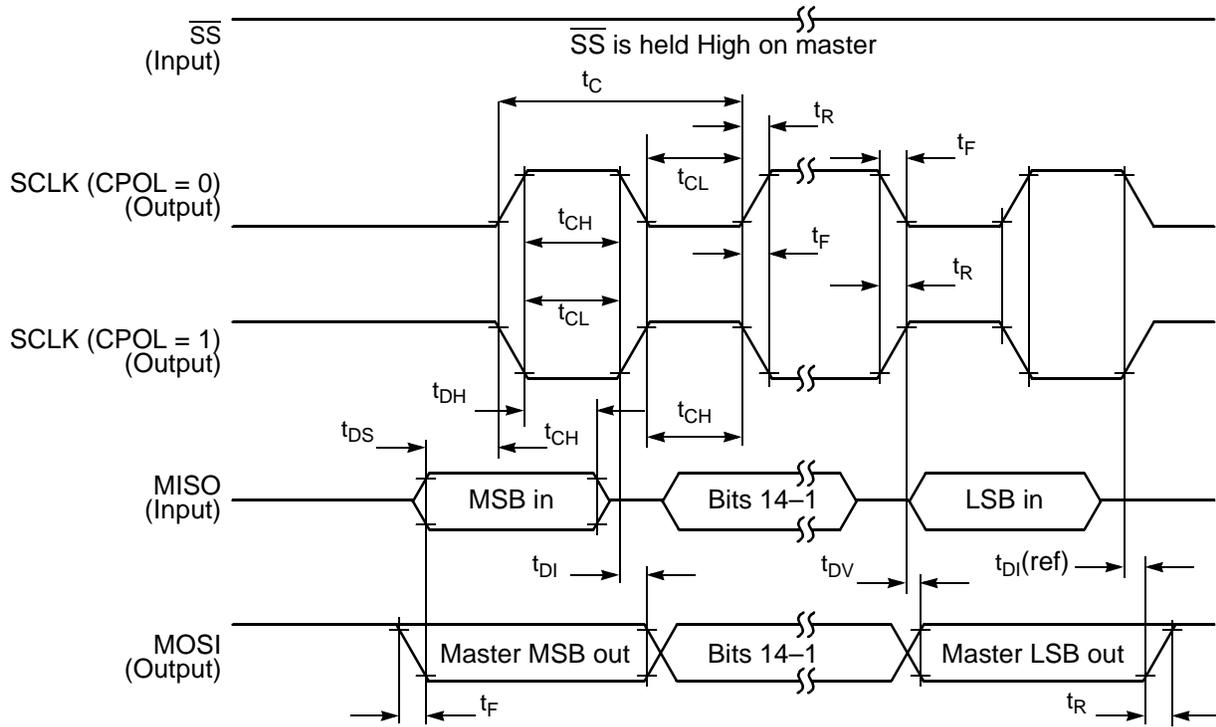
Figure 24. SPI Master Timing (CPHA = 0)
