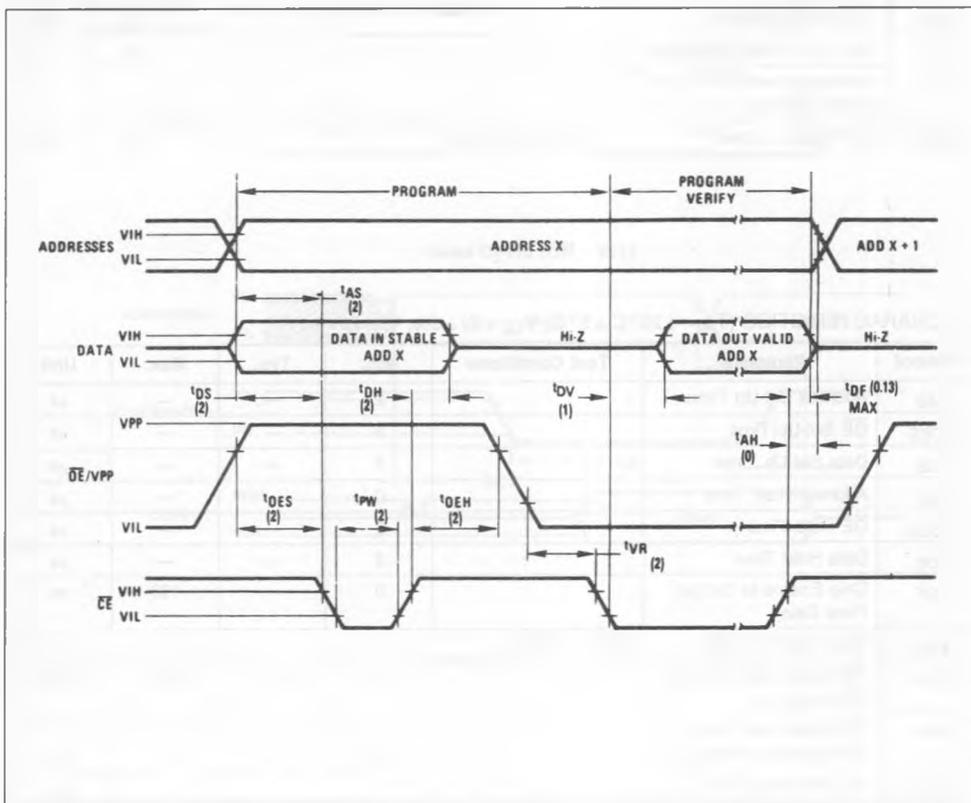
Notes: 1.  $V_{CC}$  must be applied simultaneously or before  $V_{pp}$  and removed simultaneously or after  $V_{pp}$ . The ETC 2732 must not be inserted into or removed from a board with  $V_{pp}$  at  $25 \pm 1\text{V}$  to prevent damage to the device.
