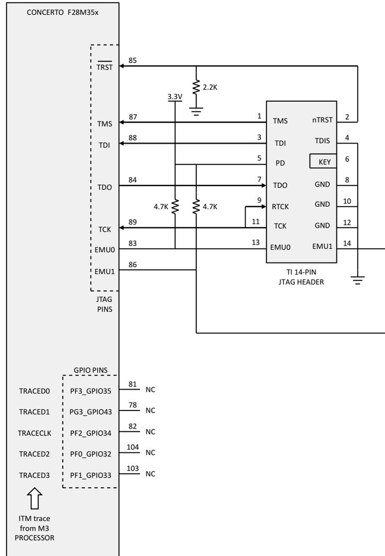
Figure 2-17. Connecting to TI 14-Pin JTAG Emulator Header
