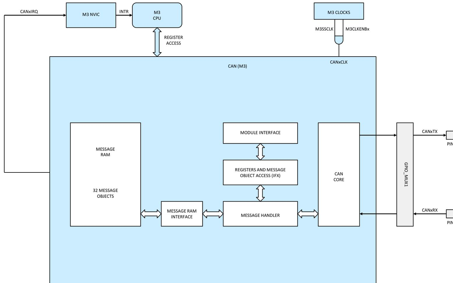
Figure 6-12. CAN (Cortex™-M3)
