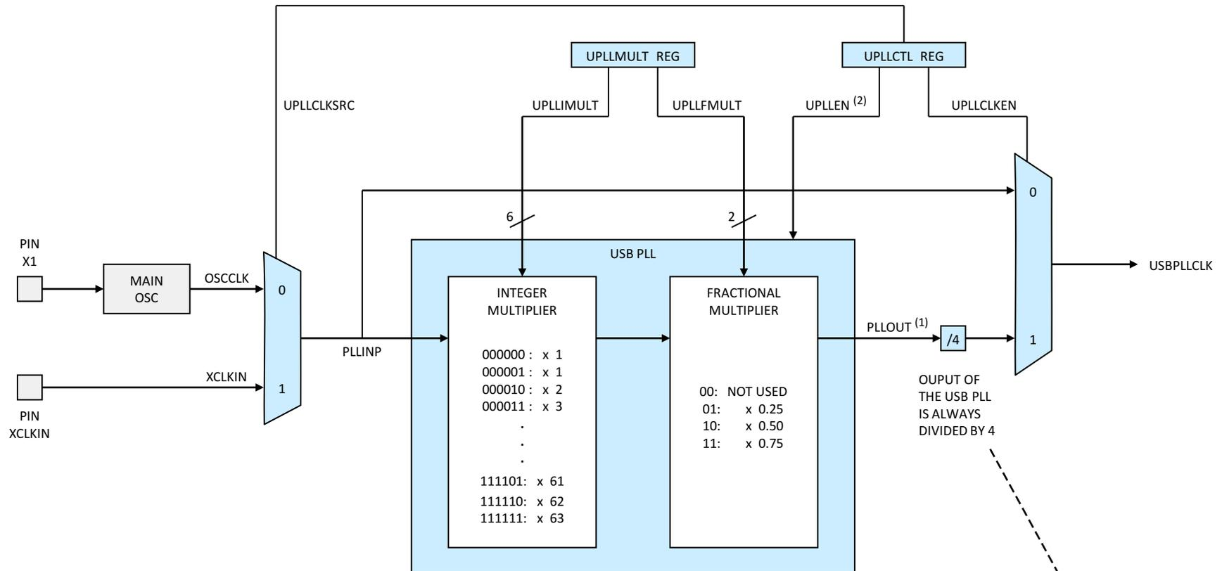
(1) OUTPUT OF THE USB PLL MUST BE ALWAYS 240MHz ( SO THAT USBPLLCLK IS 60MHz )
