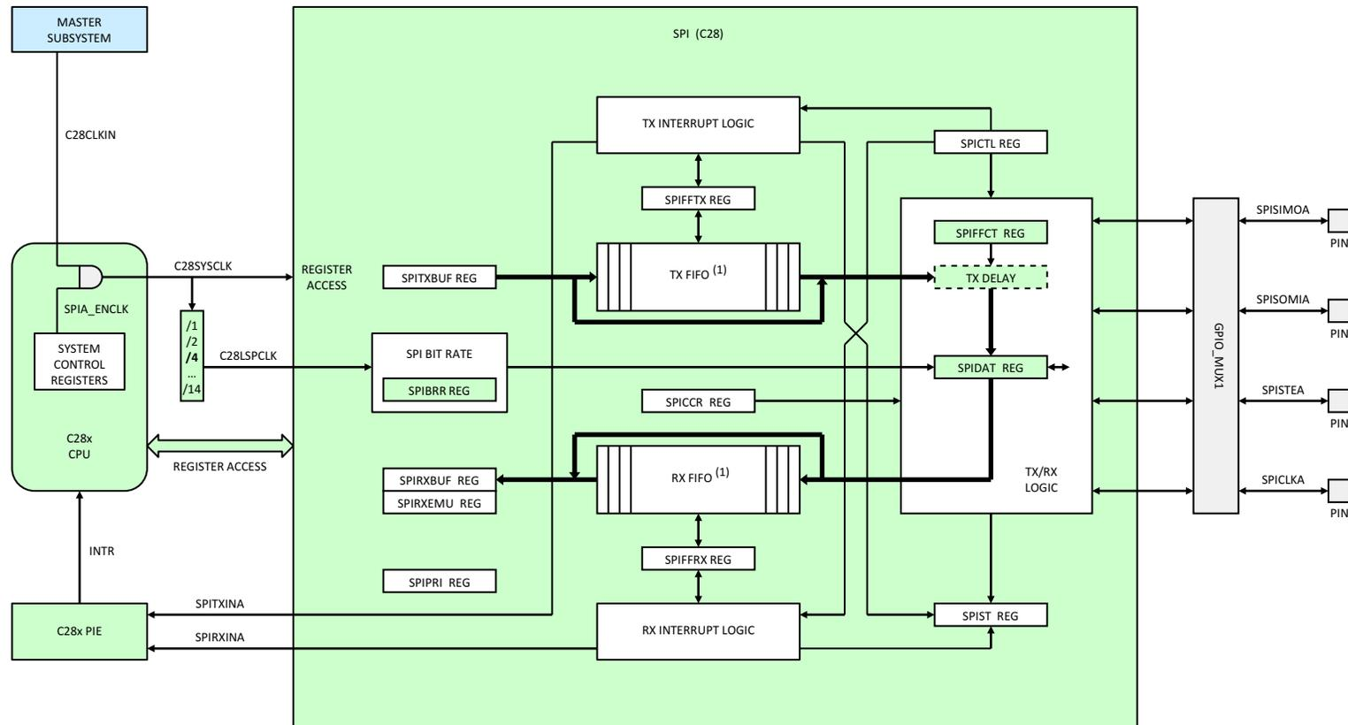
(1) RX FIFO AND TX FIFO CAN BE BYPASSED BY CONFIGURING BIT SPIFFENA OF THE SPIFFTX REGISTER
