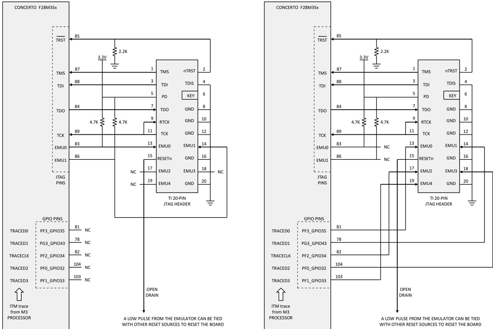
Figure 2-18. Connecting to TI 20-Pin JTAG Emulator Header
