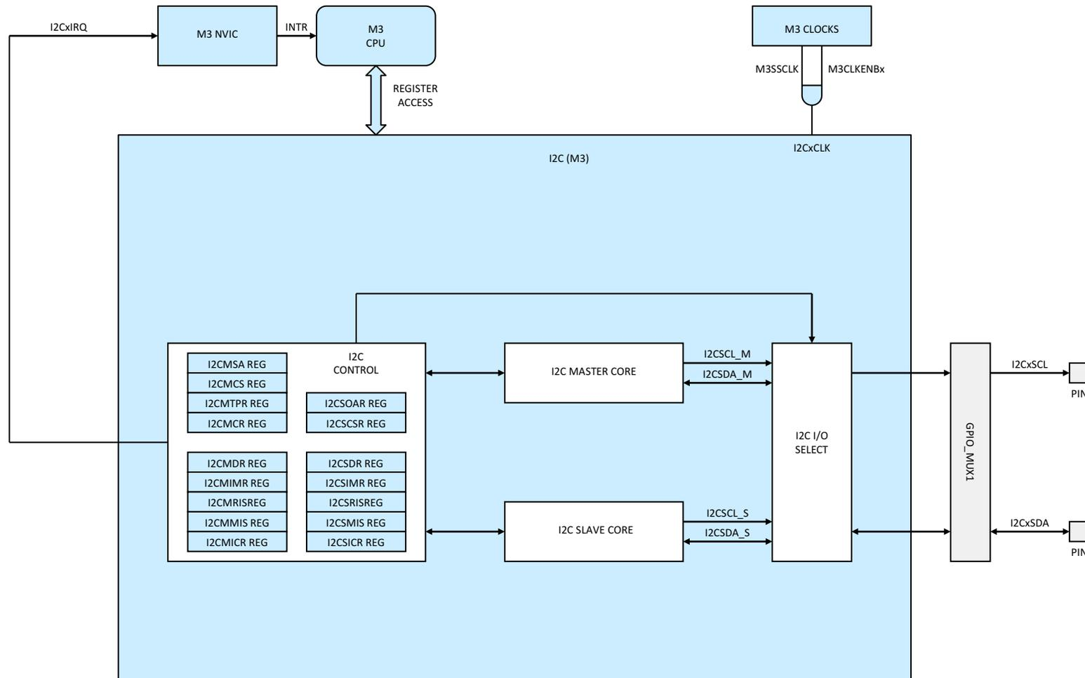
Figure 6-11. I2C (Cortex™-M3)
