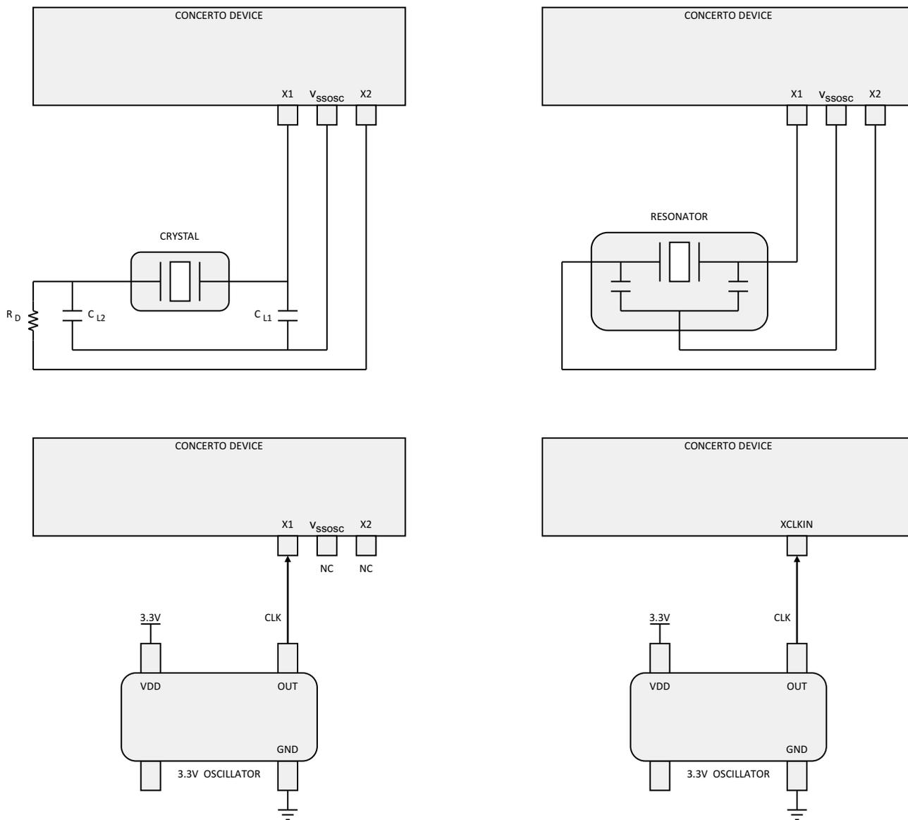
Figure 2-7. Connecting Input Clocks to a Concerto Device
