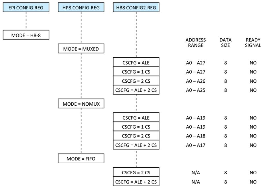
Figure 6-7. EPI 8-Bit Host Bus Mode
