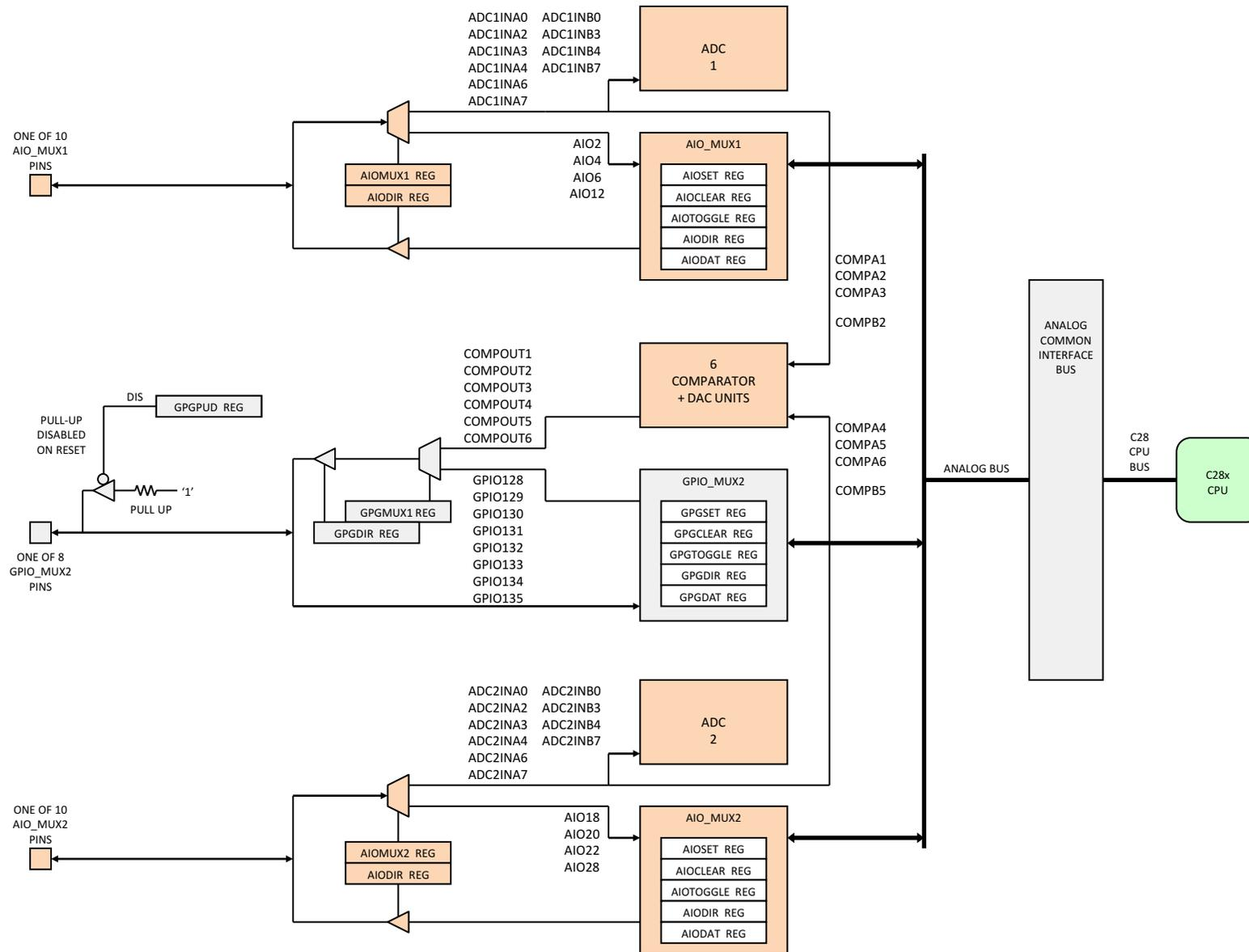
Figure 2-16. Pin Muxing on AIO\_MUX1, AIO\_MUX2, and GPIO\_MUX2
