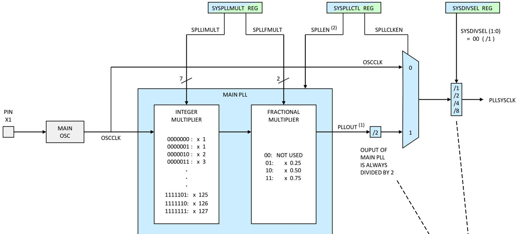
(1) OUTPUT OF THE MAIN PLL MUST RANGE BETWEEN 110- 550 MHz
