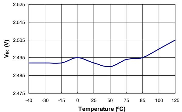
Figure 11. Reference Voltage ( $V_{IR}$ ) vs. Temperature
