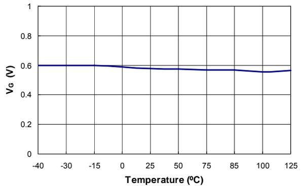
Figure 17. Green Mode Ending Voltage on COMV Pin (V<sub>G</sub>) vs. Temperature
