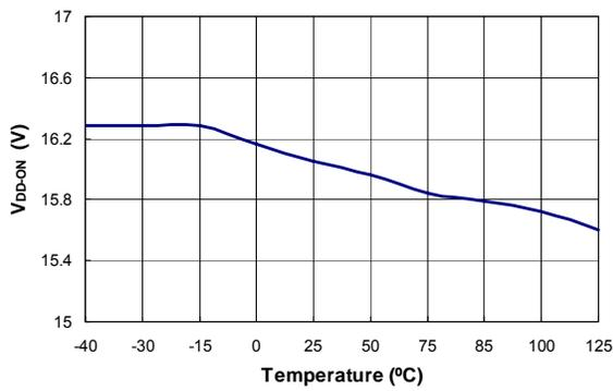
Figure 6. Turn-On Threshold Voltage ( $V_{DD-ON}$ ) vs. Temperature
