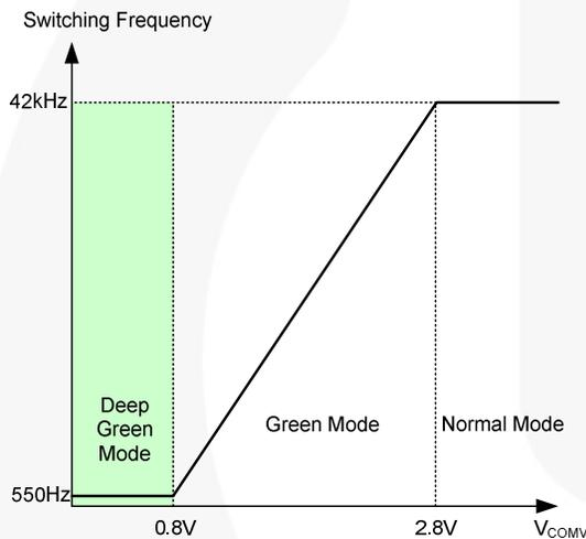
Figure 25. Switching Frequency in Green Mode
