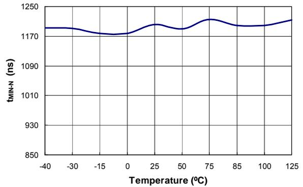
Figure 15. Minimum On Time at No Load (t<sub>MIN-N</sub>) vs. Temperature
