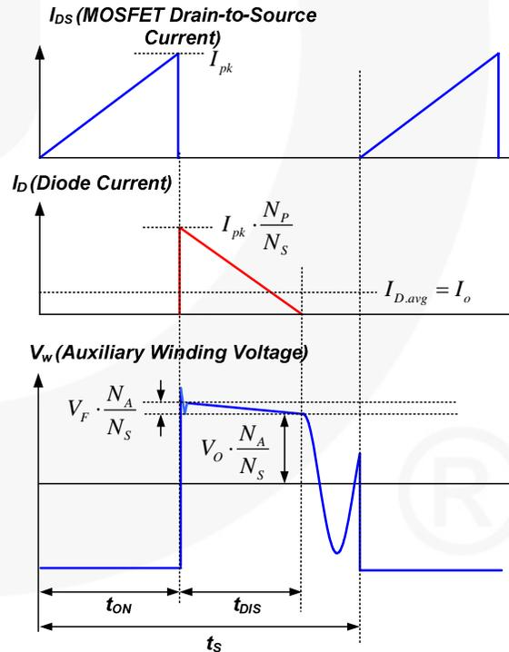
Figure 24. Key Waveforms of DCM Flyback Converter
