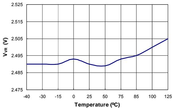
Figure 10. Reference Voltage ( $V_{VR}$ ) vs. Temperature
