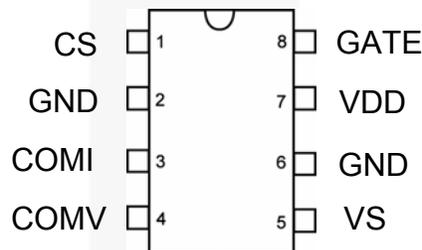
Figure 5. Pin Configuration
