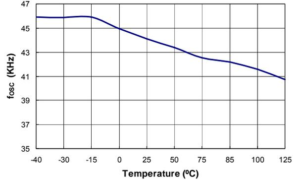
Figure 9. Center Frequency ( $f_{osc}$ ) vs. Temperature
