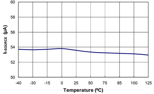
Figure 21. Output Source Current ( $I_{I-SOURCE}$ ) vs. Temperature
