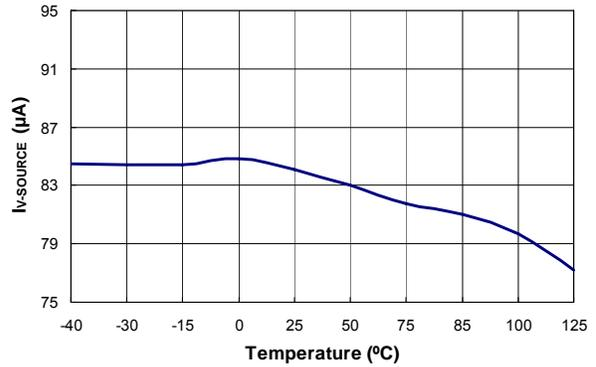
Figure 19. Output Source Current ( $I_{V-SOURCE}$ ) vs. Temperature
