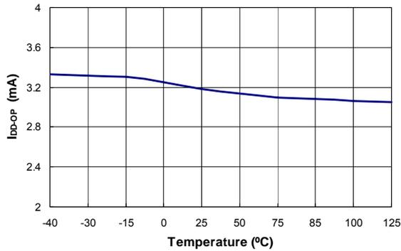
Figure 8. Operating Current ( $I_{DD-OP}$ ) vs. Temperature
