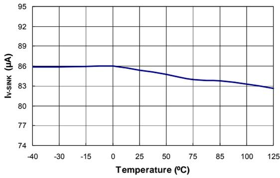
Figure 18. Output Sink Current ( $I_{V-SINK}$ ) vs. Temperature
