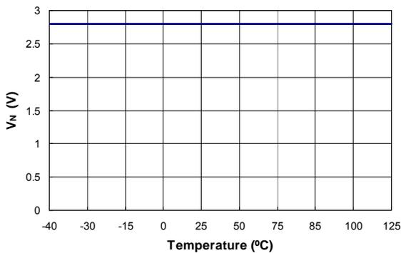
Figure 16. Green Mode Starting Voltage on COMV Pin (V<sub>N</sub>) vs. Temperature
