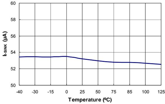
Figure 20. Output Sink Current ( $I_{I-SINK}$ ) vs. Temperature
