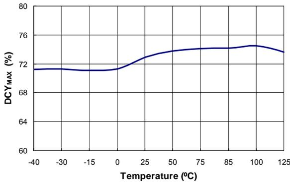
Figure 22. Maximum Duty Cycle ( $DCY_{MAX}$ ) vs. Temperature
