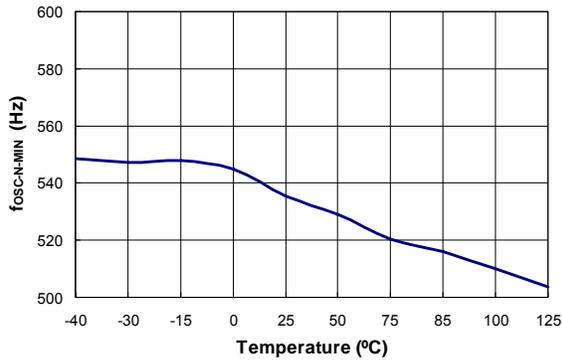
Figure 12. Minimum Frequency at No Load (f<sub>osc-N-MIN</sub>) vs. Temperature
