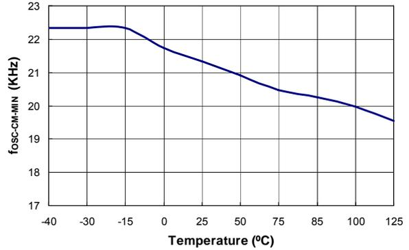
Figure 13. Minimum Frequency at CCM (f<sub>osc-CM-MIN</sub>) vs. Temperature
