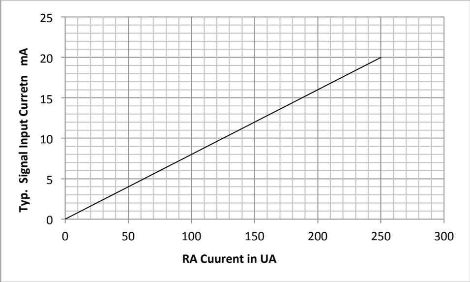
Figure 6: Interrelationship between Signal Input Current and IRA
