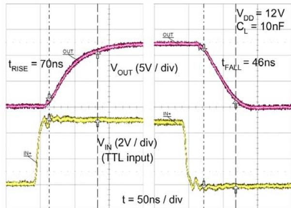
Figure 36. Rise / Fall Waveforms with 10nF Load
