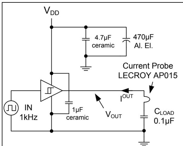
Figure 41. Quasi-Static  $I_{OUT} / V_{OUT}$  Test Circuit
