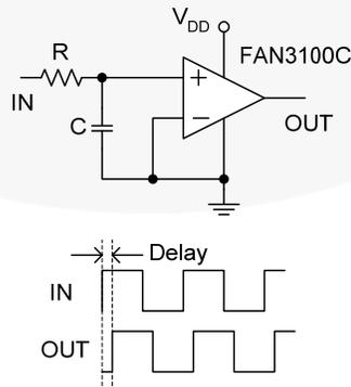
Figure 52. Programmable Time Delay Using CMOS Input
