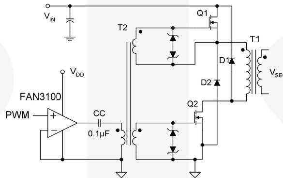
Figure 50. Driver for Two-Transistor Forward Converter Gate Transformer
