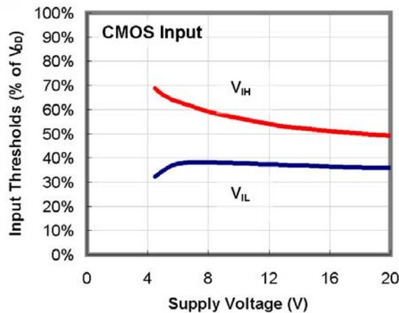
Figure 19. Input Thresholds % vs. Supply Voltage
