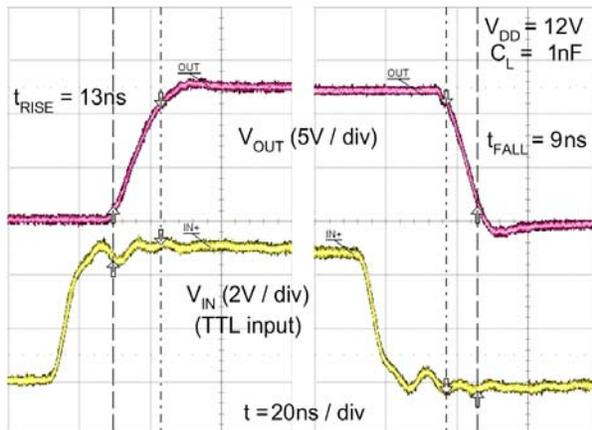
Figure 35. Rise / Fall Waveforms with 1nF Load
