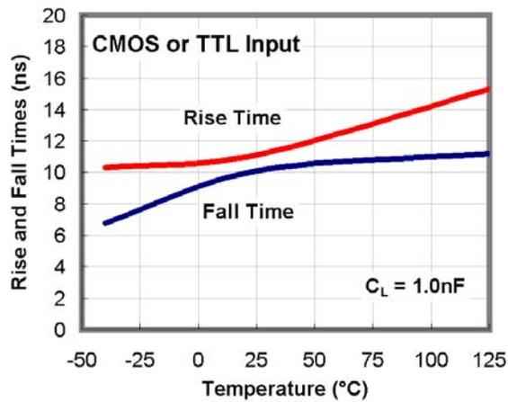
Figure 34. Rise and Fall Time vs. Temperature
