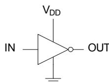
**Figure 48. Inverting Configuration**
