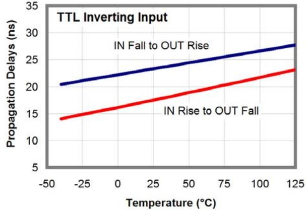
Figure 34. Propagation Delays vs. Temperature
