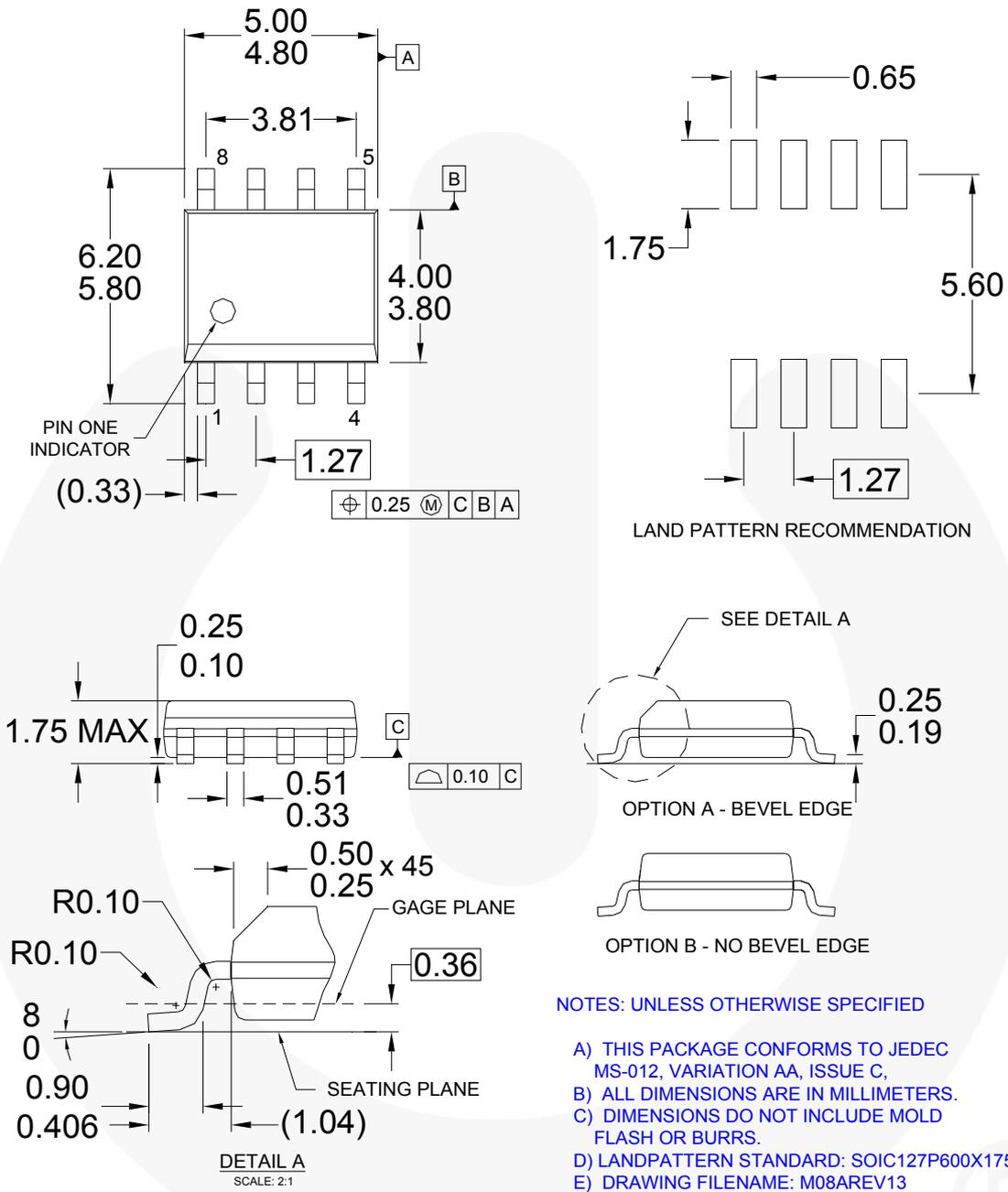
Figure 54. 8-Lead SOIC
