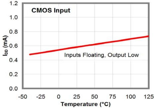
Figure 15.  $I_{DD}$  (Static) vs. Temperature<sup>(13)</sup>
