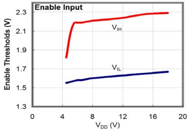
Figure 20. Enable Thresholds vs. Supply Voltage
