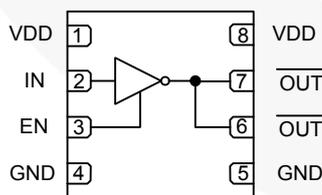
Figure 1. FAN3121 Pin Configuration
