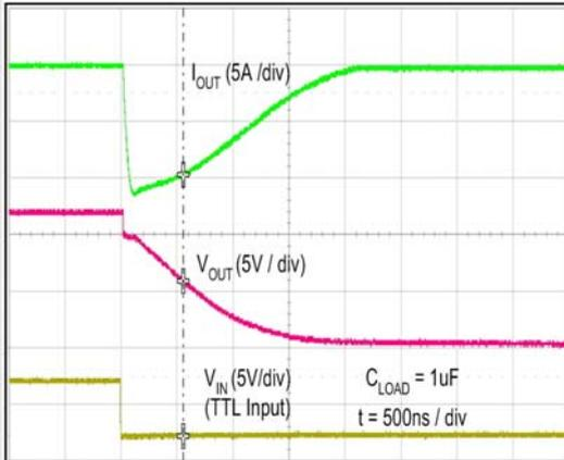
Figure 41. Quasi-Static Sink Current with  $V_{DD}=12V$ <sup>(14)</sup>
