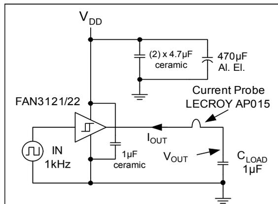
Figure 44. Quasi-Static  $I_{OUT} / V_{OUT}$  Test Circuit
