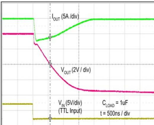
Figure 43. Quasi-Static Sink Current with  $V_{DD}=8V$ <sup>(14)</sup>
