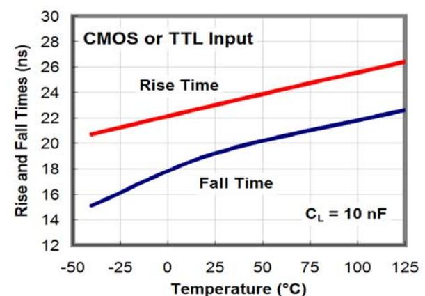
Figure 38. Rise and Fall Time vs. Temperature
