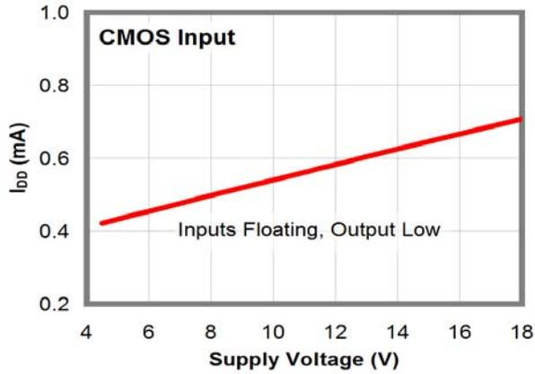
Figure 9.  $I_{DD}$  (Static) vs. Supply Voltage<sup>(13)</sup>
