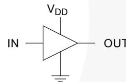
**Figure 50. Non-Inverting Driver**
