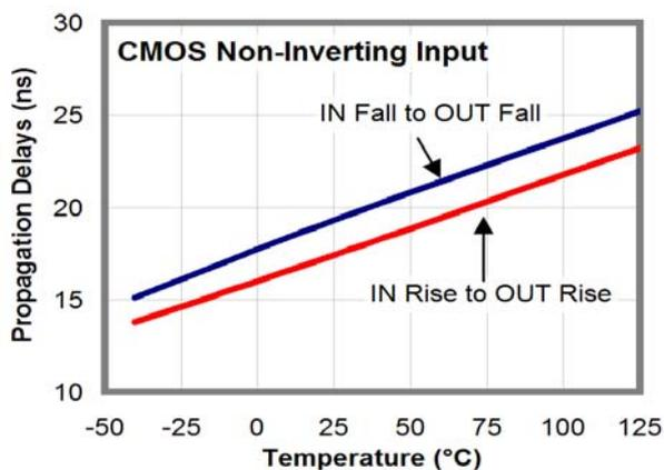
Figure 31. Propagation Delays vs. Temperature
