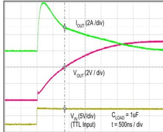
Figure 42. Quasi-Static Source Current with  $V_{DD}=8V$ <sup>(14)</sup>
