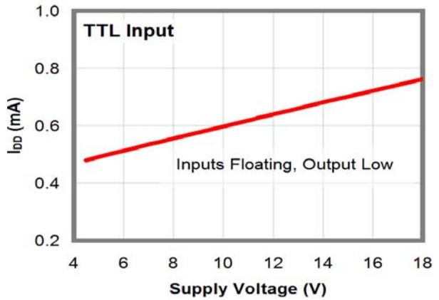
Figure 10.  $I_{DD}$  (Static) vs. Supply Voltage<sup>(13)</sup>
