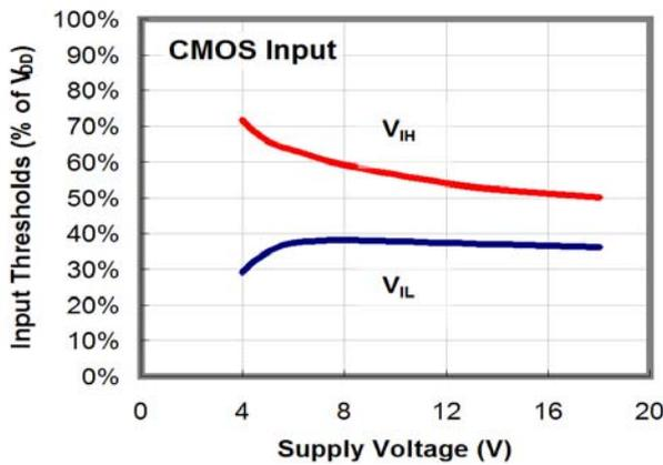
Figure 19. Input Thresholds % vs. Supply Voltage
