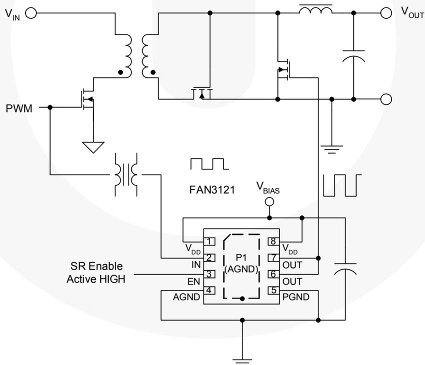
Figure 53. Hybrid Synchronous Rectification in a Forward Converter
