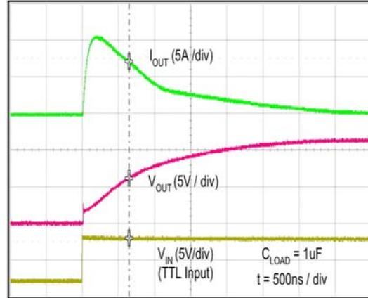
Figure 40. Quasi-Static Source Current with  $V_{DD}=12V$ <sup>(14)</sup>
