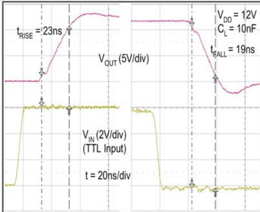
Figure 39. Rise / Fall Waveforms with 10nF Load
