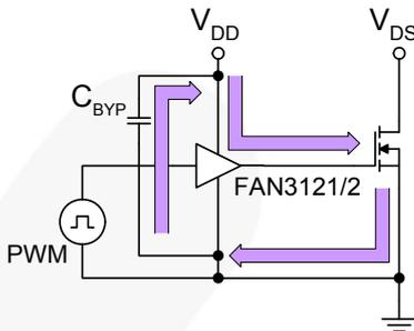
**Figure 46. Current Path for MOSFET Turn-On**
