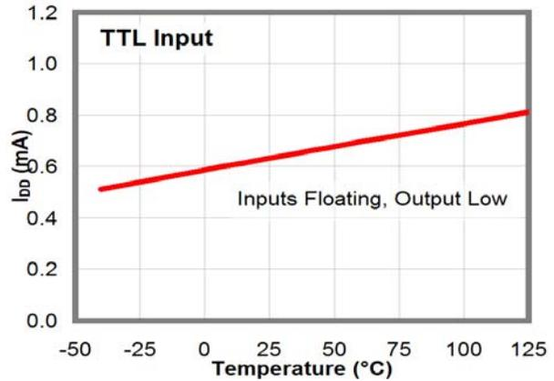
Figure 16.  $I_{DD}$  (Static) vs. Temperature<sup>(13)</sup>
