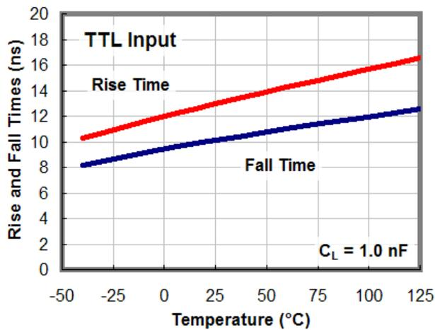
Figure 21. Rise and Fall Times vs. Temperature
