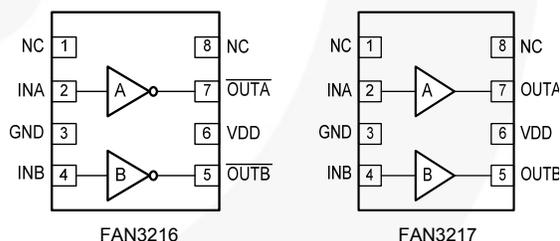
Figure 1. Pin Configurations
