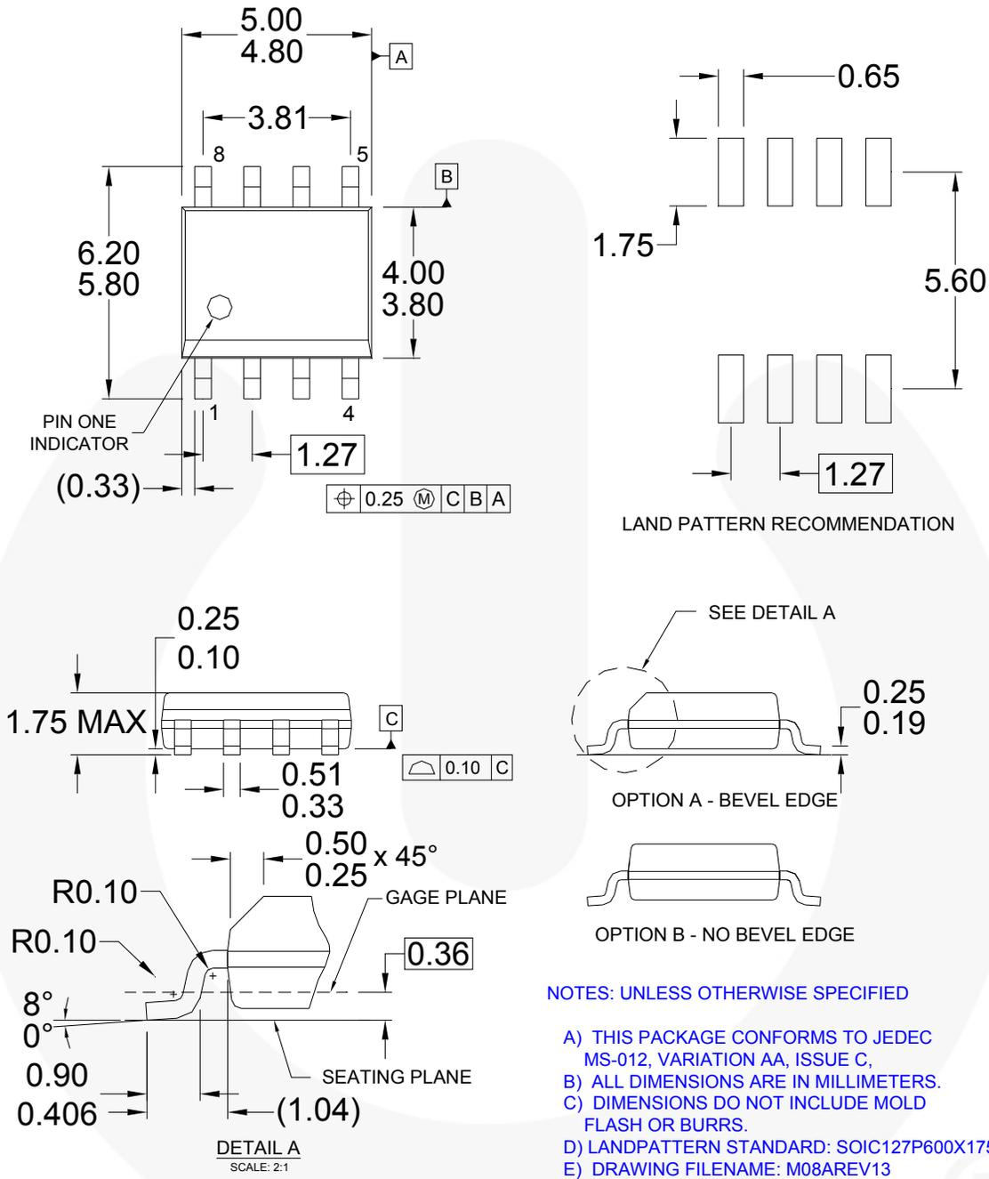
Figure 37. 8-Lead Small Outline Integrated Circuit (SOIC)
