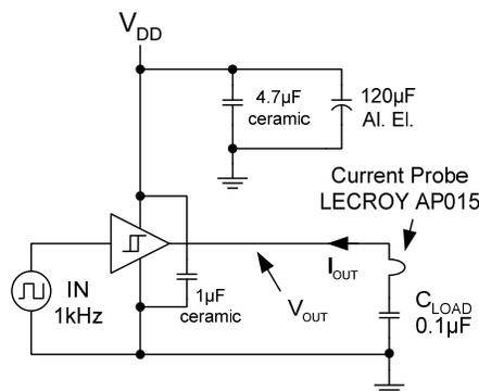
Figure 28. Quasi-Static  $I_{OUT} / V_{OUT}$  Test Circuit
