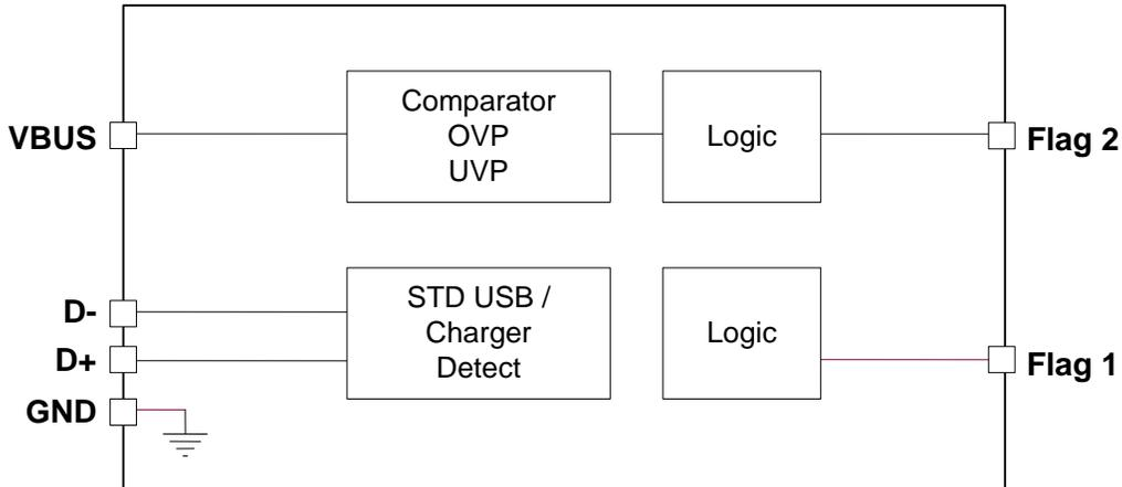
Figure 1. Block Diagram
