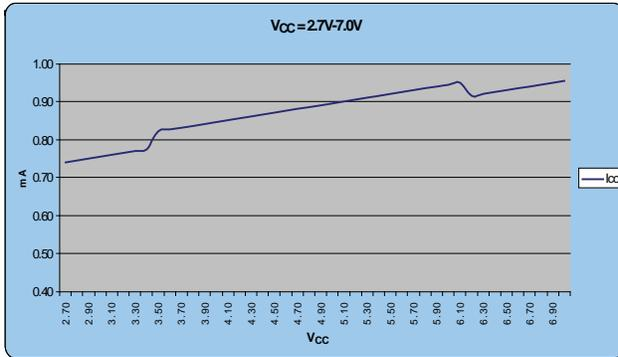
Figure 3. I<sub>Bus</sub> vs. V<sub>Bus</sub> (2.7 V-7.0 V) No Load
