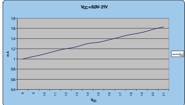
Figure 4. I<sub>Bus</sub> vs. V<sub>Bus</sub> (8.0V-21 V) No Load
