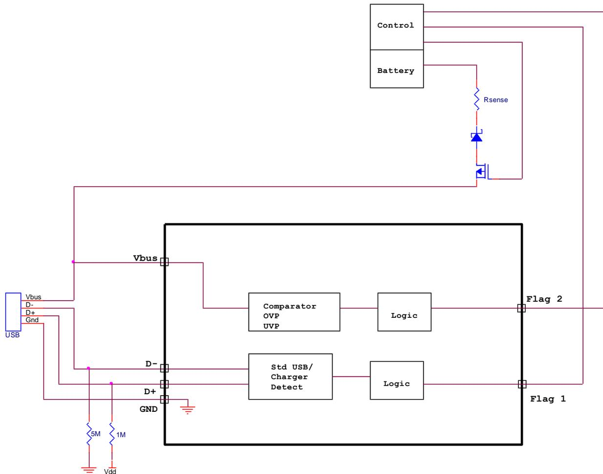
Figure 8. Typical System Application without USB Transceiver
