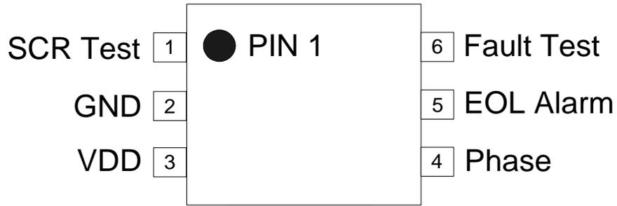
Figure 3. Pin Assignments
