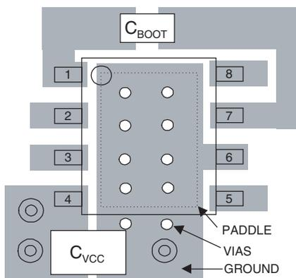
**Figure 7. Recommended layout for MLP package.
