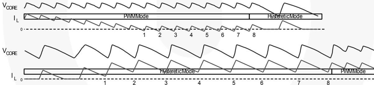
Figure 11. Transitioning Between PWM and Hysteretic Mode
