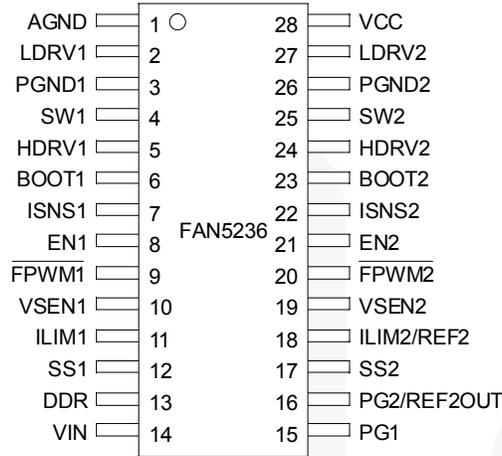
Figure 3. Pin Configuration
