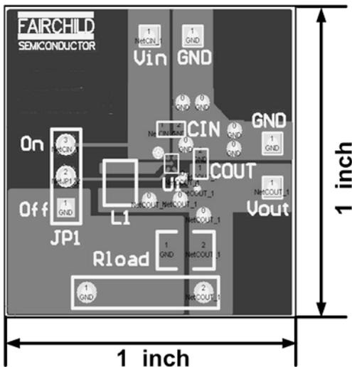
**Figure 7. The FAN5350 Evaluation Board PCB (CSP)**
