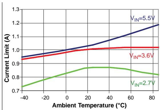
Figure 16. PMOS Current Limit in Closed Loop
