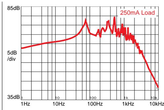
Figure 18. Power Supply Rejection Ratio in CCM
