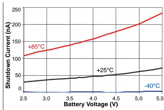
Figure 17. Shutdown Supply Current vs. Battery Voltage
