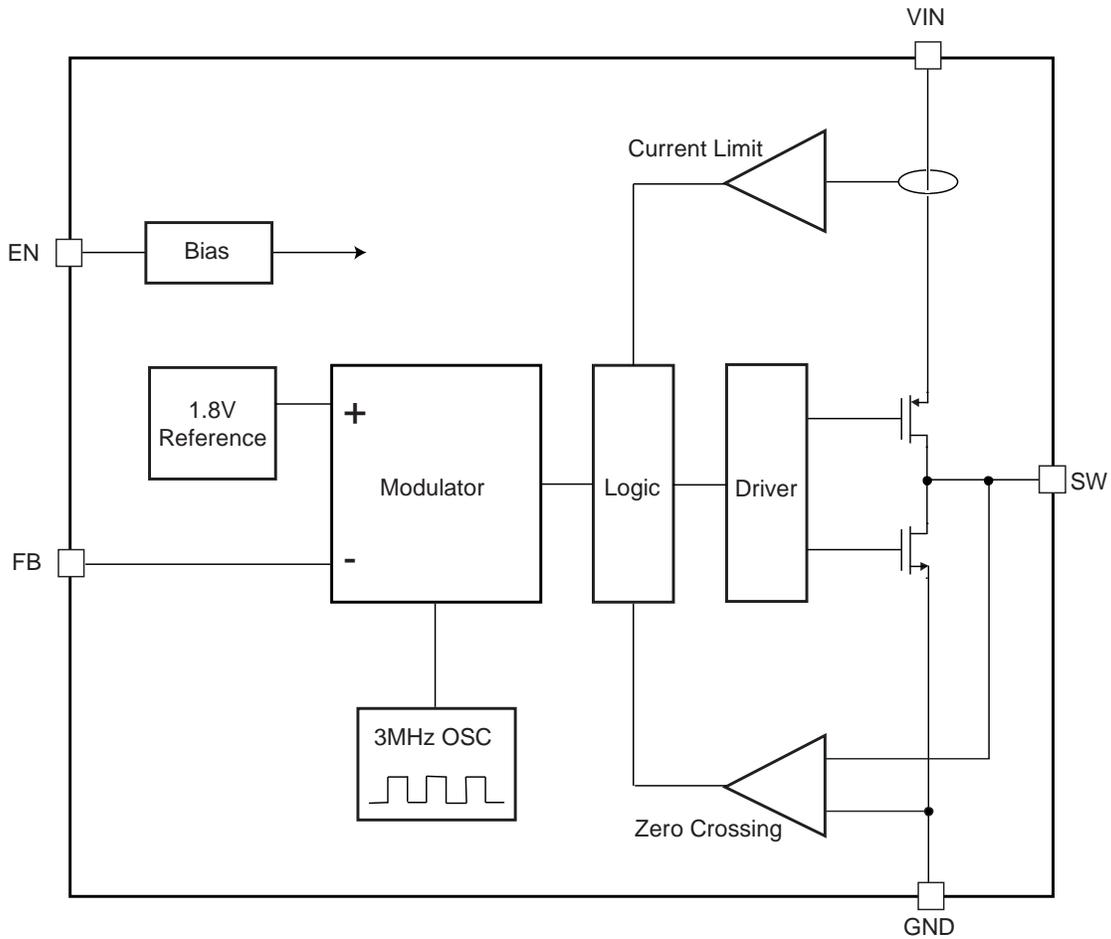
Figure 3. Block Diagram
