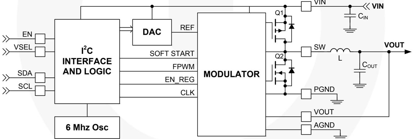
Figure 3 Block Diagram
