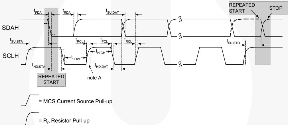
Note A: First rising edge of SCLH after Repeated Start and after each ACK bit.
