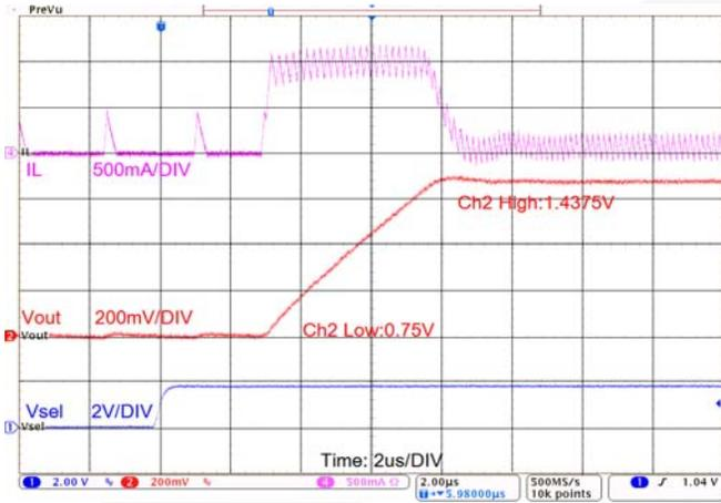
Figure 23. VSEL Transition, Single Step (DefSlew = 7),  $R_{LOAD} = 24\Omega$
