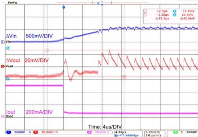
**Figure 19. Combined Line/Load Transient 3.0 to 3.6V<sub>IN</sub> Combined with 500 to 50mA Load Transient**
