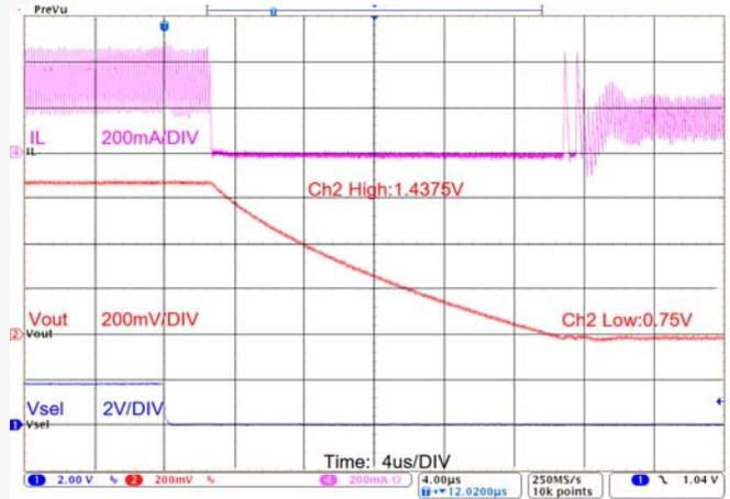
Figure 28. VSEL Transition, VSEL 1 to 0,  $R_{LOAD} = 4\Omega$
