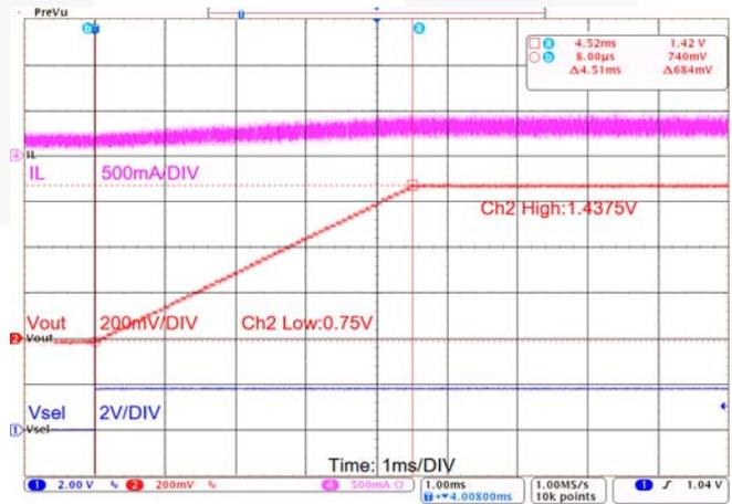
Figure 26. VSEL Transition, DefSlew = 0,  $R_{LOAD} = 4\Omega$
