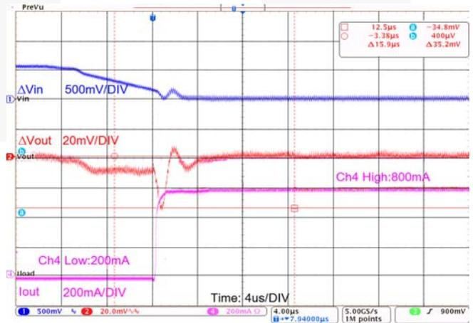
**Figure 22. Combined Line/Load Transient 3.6 to 3.0V<sub>IN</sub> Combined with 200 to 800mA Load Transient**
