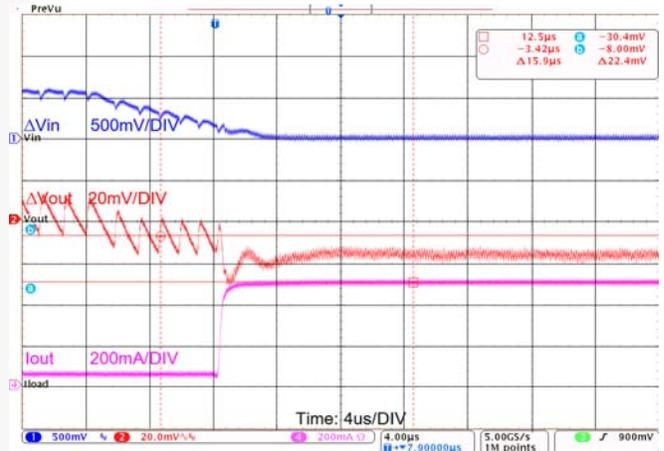
**Figure 20. Combined Line/Load Transient 3.6 to 3.0V<sub>IN</sub> Combined with 50 to 500mA Load Transient**
