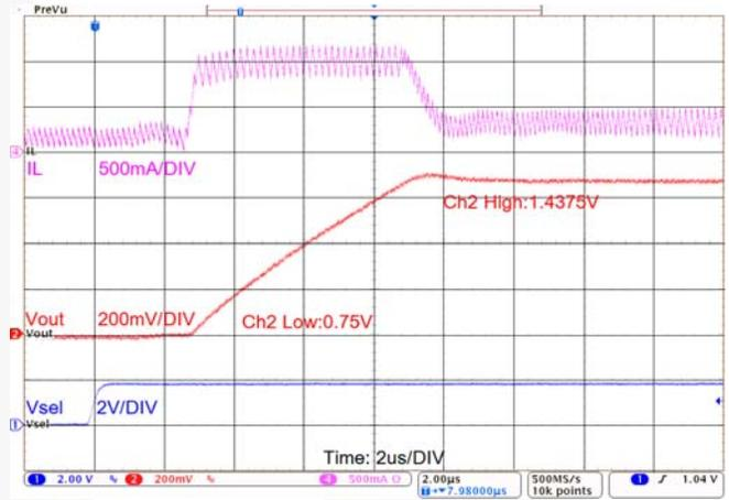
Figure 24. VSEL Transition, Single Step (DefSlew = 7),  $R_{LOAD} = 4\Omega$
