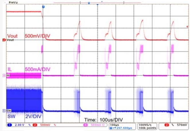
Figure 32. Over-Current Fault Response,  $R_{LOAD} = 500m\Omega$
