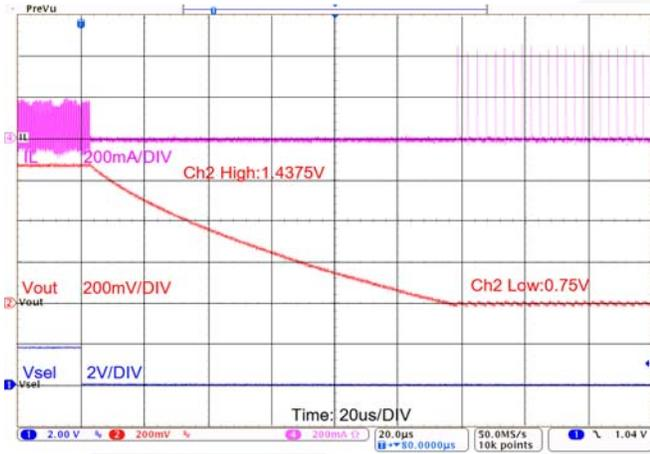
Figure 27. VSEL Transition, VSEL 1 to 0,  $R_{LOAD} = 24\Omega$
