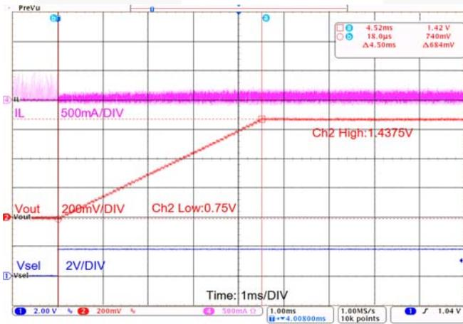
Figure 25. VSEL Transition, DefSlew = 0,  $R_{LOAD} = 24\Omega$
