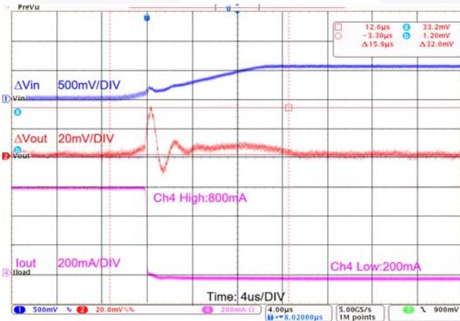
**Figure 21. Combined Line/Load Transient 3.0 to 3.6V<sub>IN</sub> Combined with 800 to 200mA Load Transient**
