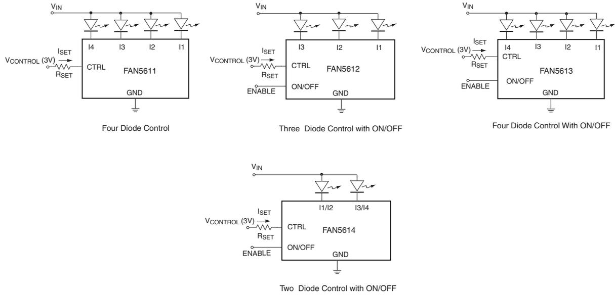
Figure 1. Typical Applications for FAN5611, FAN5612, FAN5613, FAN5614
