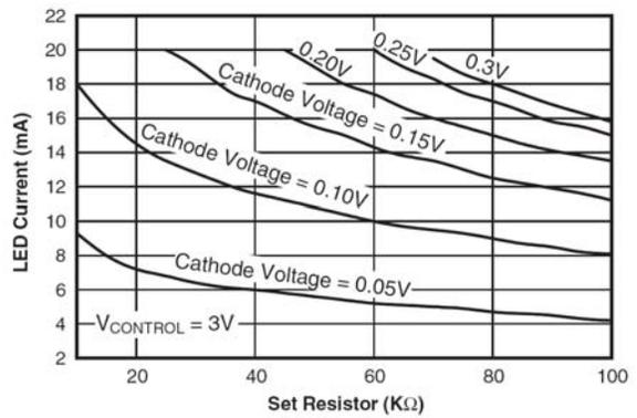
**Figure 8. FAN5614 LED Current vs. Set Resistor**
