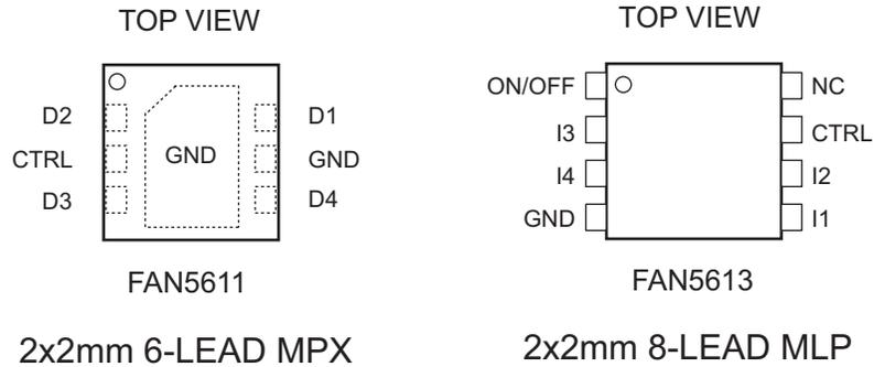
Figure 2. Pin Assignments for FAN5611, FAN5612, FAN5613, FAN5614
