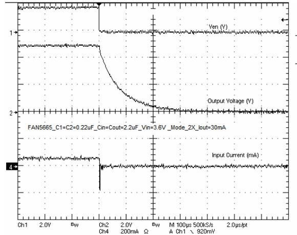
**Figure 30. Turn-off at  $I_{OUT} = 30mA$  in 2x Mode**
