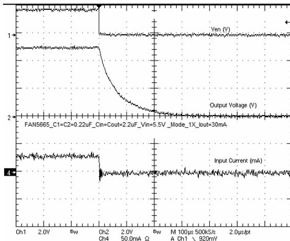
Figure 26. Turn-off at  $I_{OUT} = 30\text{mA}$  in 1x Mode
