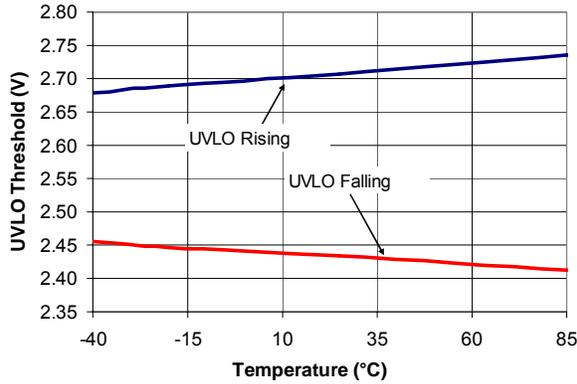
**Figure 9. UVLO Threshold vs. Temperature**
