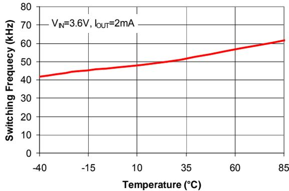
**Figure 5. Light-Load Switching Frequency vs. Temperature**
