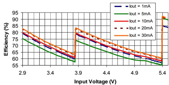
**Figure 15. Efficiency vs. Input Voltage**
