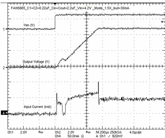
Figure 27. Start-up at  $I_{OUT} = 30\text{mA}$  in 1.5x Mode
