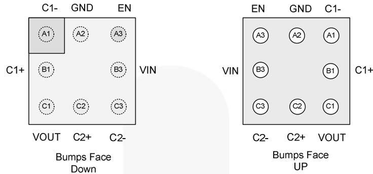
Figure 2. Pin Configuration
