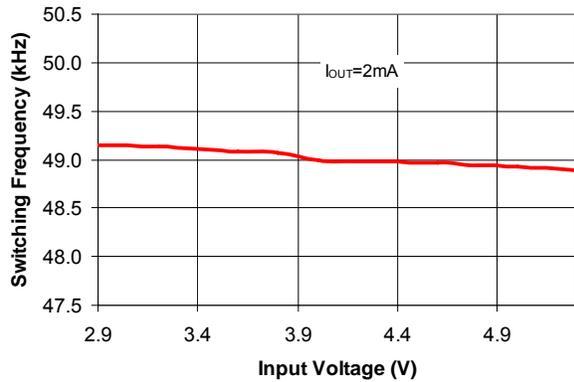
**Figure 3. Light-Load Switching Frequency vs. Input Voltage**
