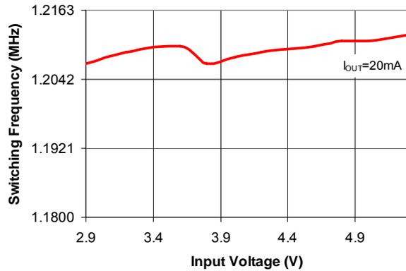
**Figure 4. Heavy-Load Switching Frequency vs. Input Voltage**
