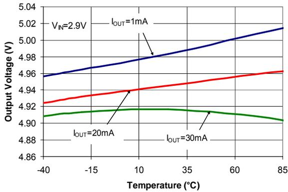
**Figure 11. Output Voltage vs. Temperature**
