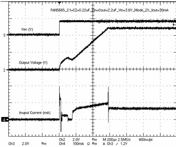
**Figure 29. Start-up at  $I_{OUT} = 30mA$  in 2x Mode**
