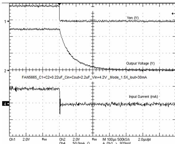
Figure 28. Turn-off at  $I_{OUT} = 30\text{mA}$  in 1.5x Mode
