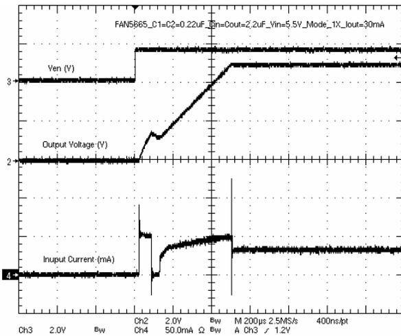
Figure 25. Start-up at  $I_{OUT} = 30\text{mA}$  in 1x Mode
