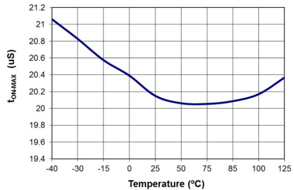
Figure 22. Maximum On Time ( $t_{ON-MAX}$ ) vs. Temperature
