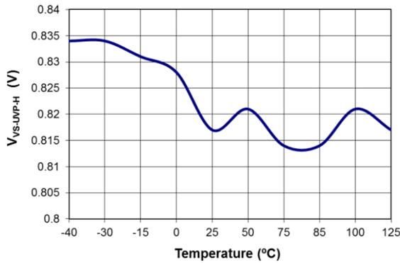
Figure 17. Output Under-Voltage Protection ( $V_{VS-UV-P-H}$ ) vs. Temperature
