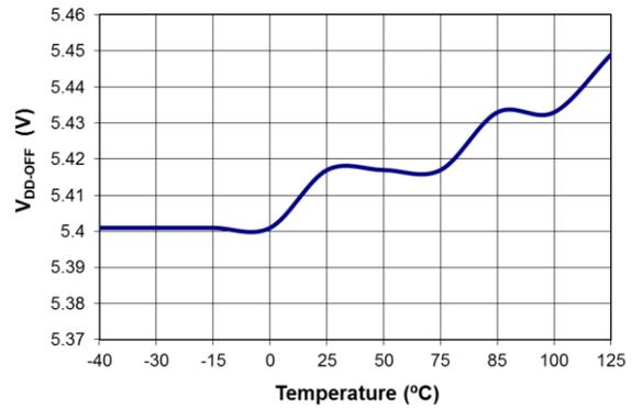
**Figure 6. Turn-Off Threshold Voltage (V<sub>DD-OFF</sub>) vs. Temperature**
