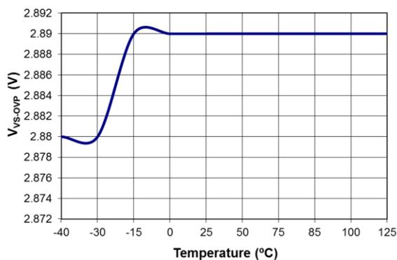
Figure 16. Output Over-Voltage-Protection ( $V_{VS-OVP}$ ) vs. Temperature
