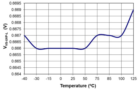
Figure 18. Output Under-Voltage Protection ( $V_{VS-UV-P-L}$ ) vs. Temperature
