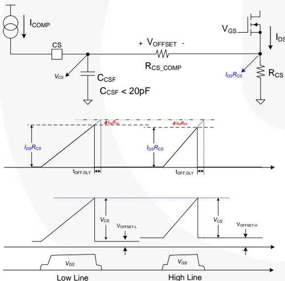
**Figure 41. Line Voltage Compensation**
