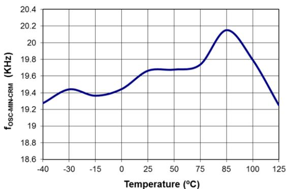
Figure 11. Minimum Frequency for CrM ( $f_{OSC-MIN-CrM}$ ) vs. Temperature
