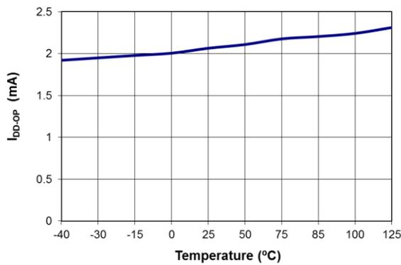
**Figure 7. Operating Supply Current (I<sub>DD-OP</sub>) vs. Temperature**
