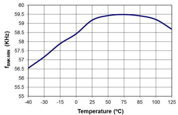
**Figure 10. Minimum Blanking Frequency (f<sub>BNK-MIN</sub>) vs. Temperature**
