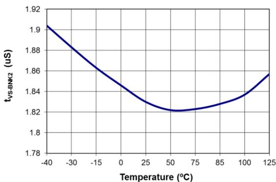
Figure 15.  $V_S$  Sampling Blanking Time 2 ( $t_{VS-BNK2}$ ) vs. Temperature
