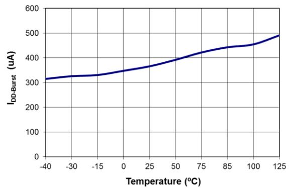
**Figure 8. Burst-Mode Operating Supply Current (I<sub>DD-Burst</sub>) vs. Temperature**
