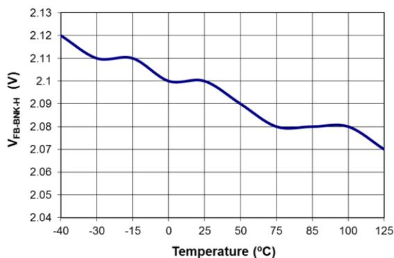
Figure 12. Frequency Fold-back Starting ( $V_{FB-BNK-H}$ ) vs. Temperature
