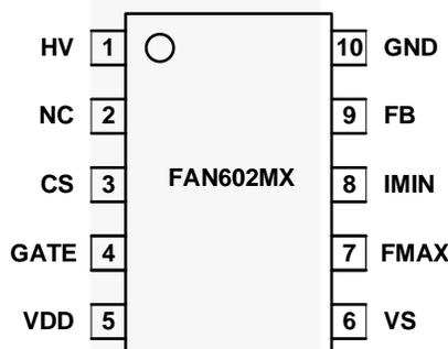
Figure 4. Pin Assignment
