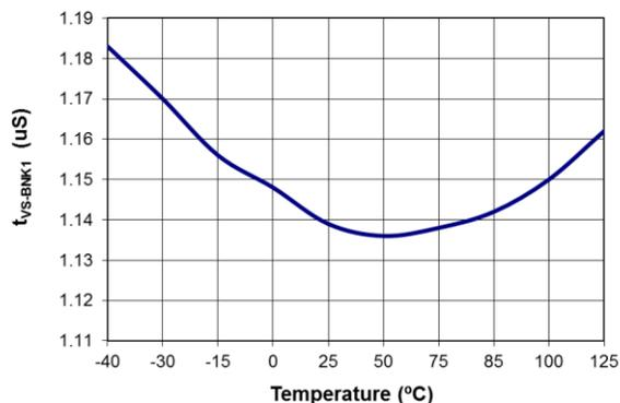
Figure 14.  $V_S$  Sampling Blanking Time 1 ( $t_{VS-BNK1}$ ) vs. Temperature
