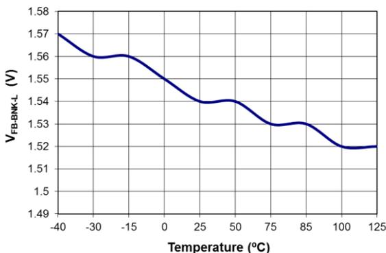
Figure 13. Frequency Fold-back Stopping ( $V_{FB-BNK-L}$ ) vs. Temperature
