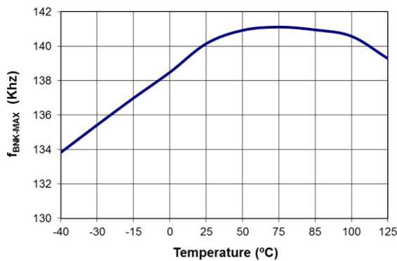
**Figure 9. Maximum Blanking Frequency (f<sub>BNK-MAX</sub>) vs. Temperature**
