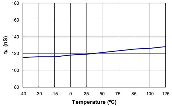
Figure 18. Rising Time (t<sub>R</sub>) vs. Temperature
