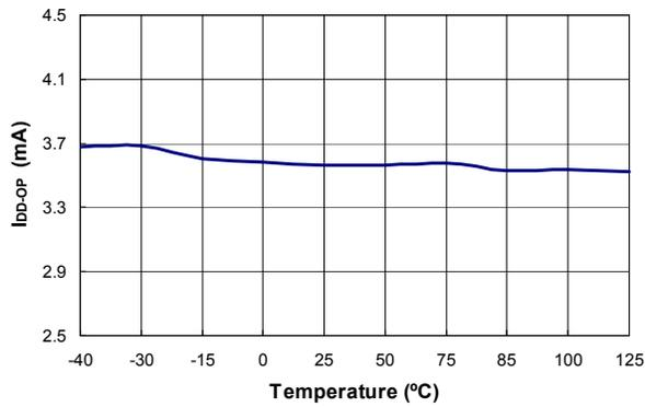
**Figure 7. Operating Current ( $I_{DD-OP}$ ) vs. Temperature**
