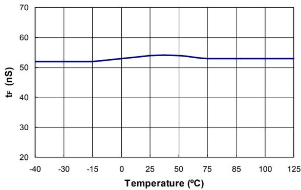
Figure 19. Falling Time (t<sub>F</sub>) vs. Temperature
