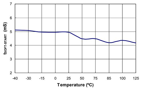
**Figure 16. Period during Startup ( $t_{SOFT-START}$ ) vs. Temperature**
