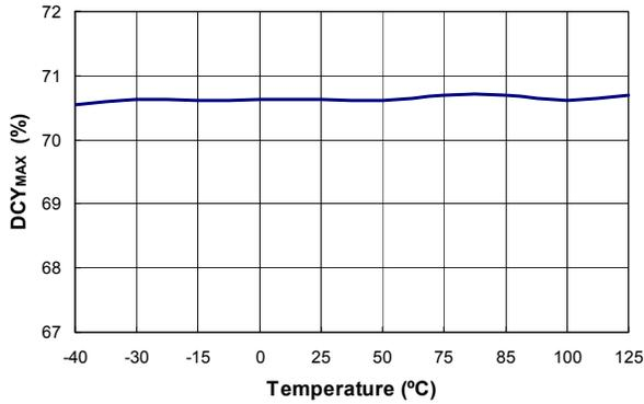
Figure 17. Maximum Duty Cycle (DCY<sub>MAX</sub>) vs. Temperature
