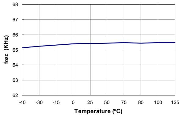
**Figure 9. Center Frequency ( $f_{OSC}$ ) vs. Temperature**
