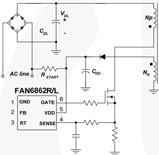
Figure 21. Startup Circuit
