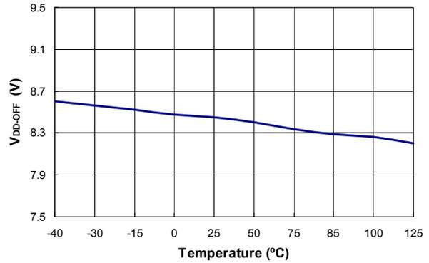
**Figure 6. Turn-Off Threshold Voltage ( $V_{DD-OFF}$ ) vs. Temperature**
