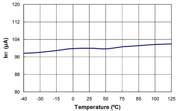
Figure 20. Output Current of RT Pin (I<sub>RT</sub>) vs. Temperature
