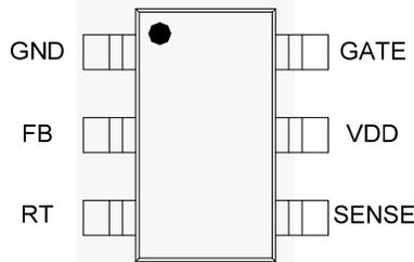
Figure 4. Pin Assignments
