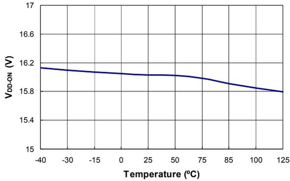
**Figure 5. Turn-On Threshold Voltage ( $V_{DD-ON}$ ) vs. Temperature**
