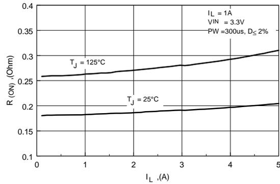
**Figure 4.  $R_{(ON)}$  Versus  $I_L$  at  $V_{IN} = 3.3V$ .**
