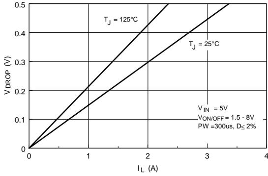
**Figure 1.  $V_{DROP}$  Versus  $I_L$  at  $V_{IN} = 5V$ .**
