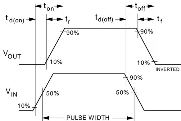
**Figure 11. Switching Waveforms.**
