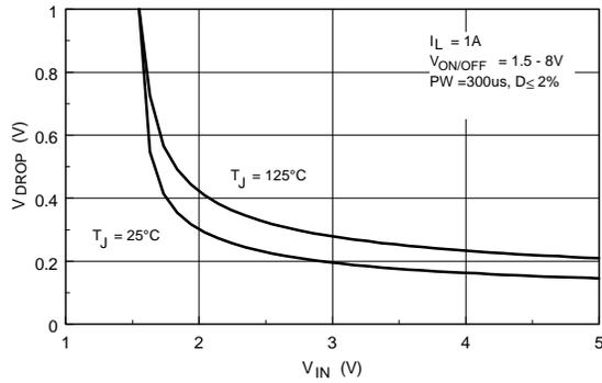
**Figure 3.  $V_{DROP}$  Versus  $V_{IN}$  at  $I_L = 1A$ .**
