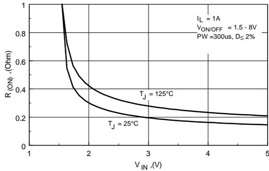
**Figure 5. On Resistance Variation with Input Voltage.**
