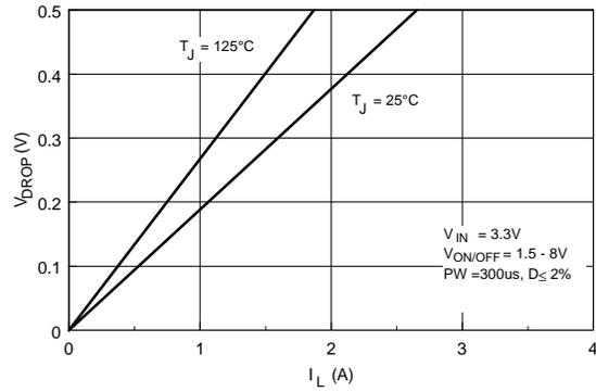
**Figure 2.  $V_{DROP}$  Versus  $I_L$  at  $V_{IN} = 3.3V$ .**
