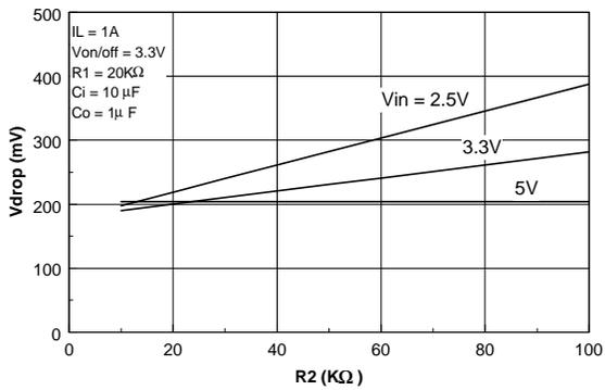
**Figure 10.  $V_{drop}$  Variation with  $V_{in}$  and  $R_2$ .**
