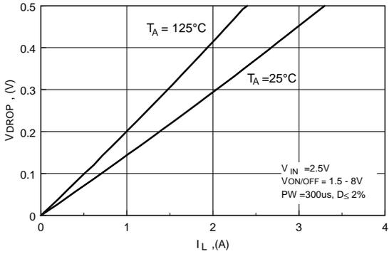
**Figure 3. Conduction Voltage Drop Variation with Load Current.**
