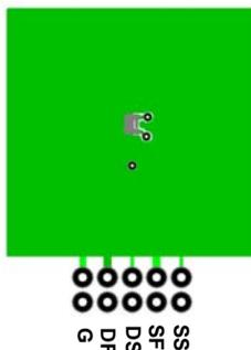
a.  $70\text{ }^\circ\text{C/W}$  when mounted on a  $1\text{ in}^2$  pad of 2 oz copper.
