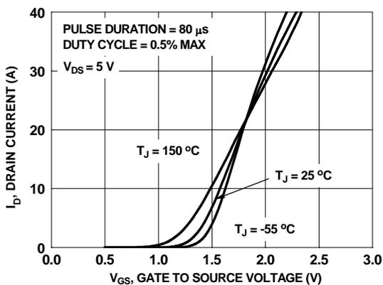
**Figure 5. Transfer Characteristics**
