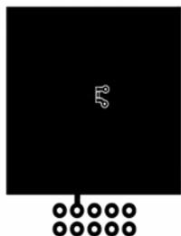
a.  $60\text{ }^\circ\text{C}/\text{W}$  when mounted on a  $1\text{ in}^2$  pad of 2 oz copper.
