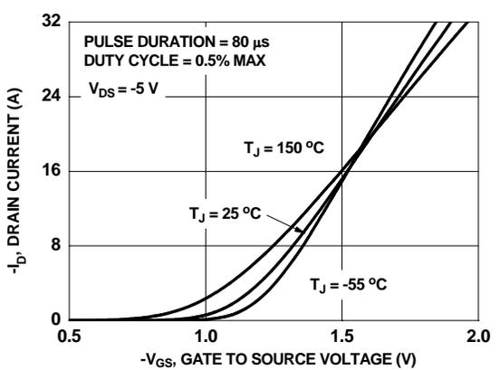
**Figure 5. Transfer Characteristics**
