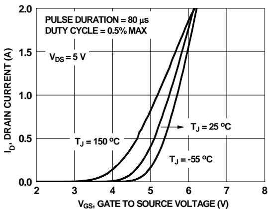
**Figure 5. Transfer Characteristics**
