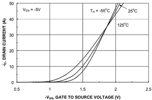
Figure 5. Transfer Characteristics.
