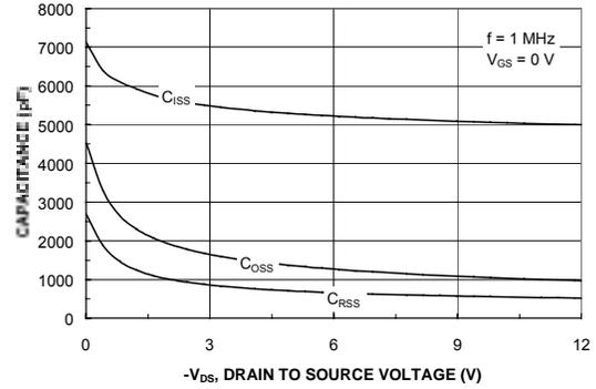
Figure 8. Capacitance Characteristics.
