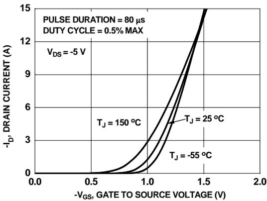
**Figure 5. Transfer Characteristics**
