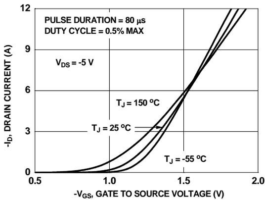
**Figure 5. Transfer Characteristics**
