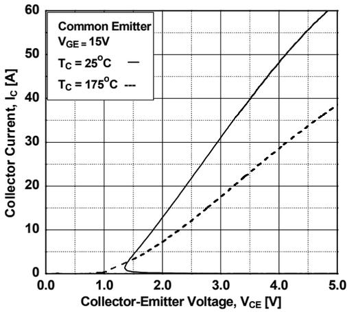
Figure 4. Transfer Characteristics
