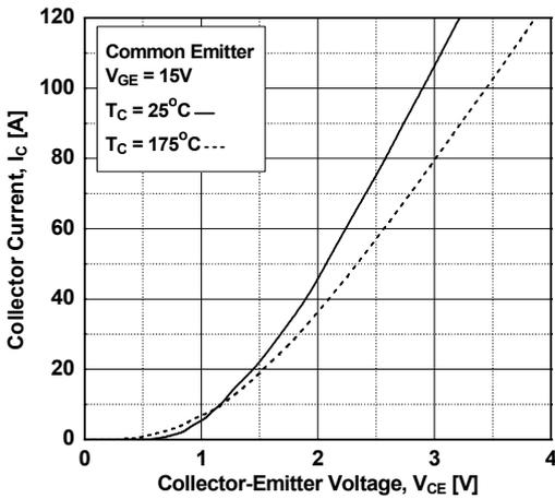
Figure 4. Transfer Characteristics
