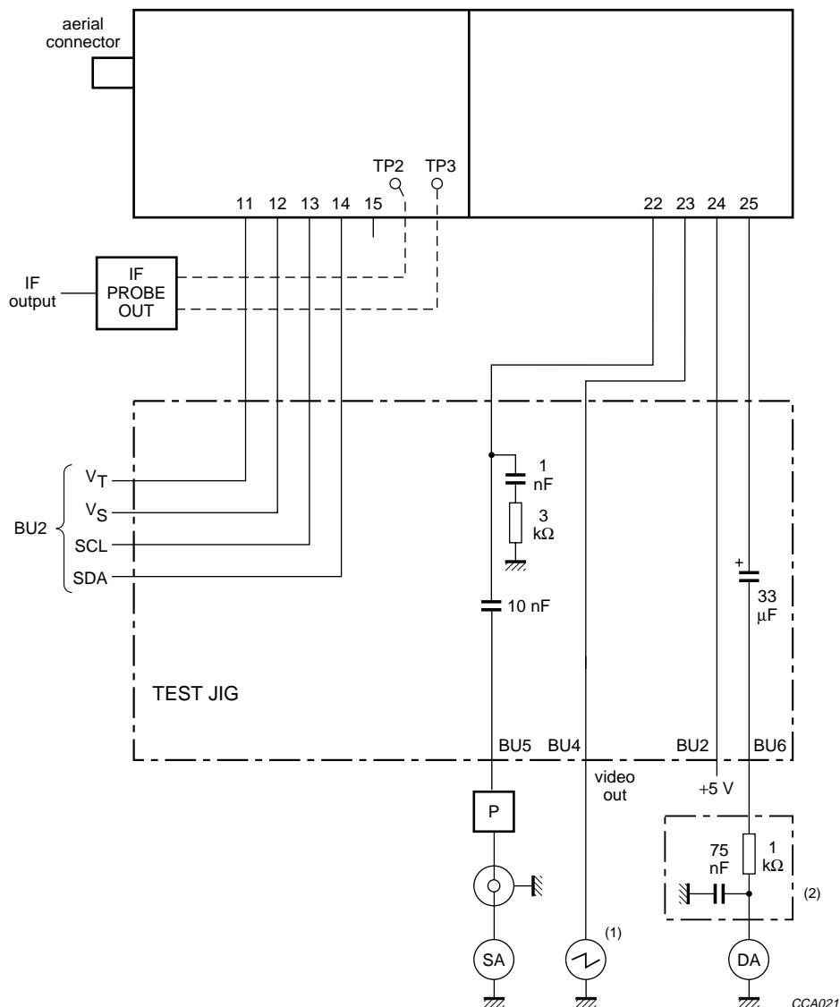
(1) BU4 loaded with  $75 \Omega$ .(2)  $75 \mu\text{s}$  de-emphasis.
