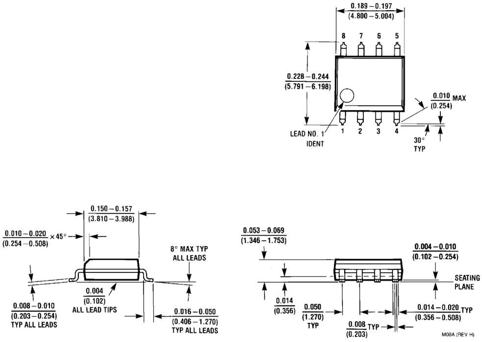
**8-Lead Small Outline Integrated Circuit (SOIC), JEDEC MS-012, 0.150" Narrow
