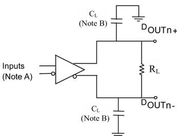
**Note A:** All LVDS input pulses have frequency = 10MHz,  $t_R$  or  $t_F <= 0.5 \text{ ns}$
