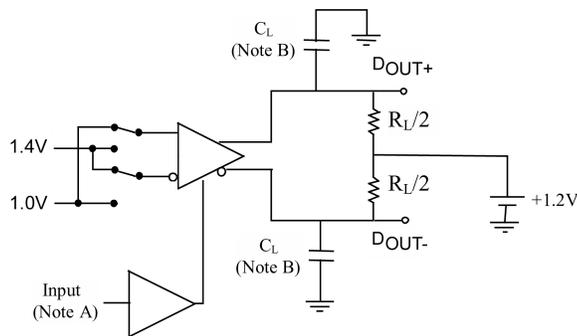
Note A: All LVTTTL input pulses have frequency = 10 MHz,  $t_r$  or  $t_f < 2 \text{ ns}$
