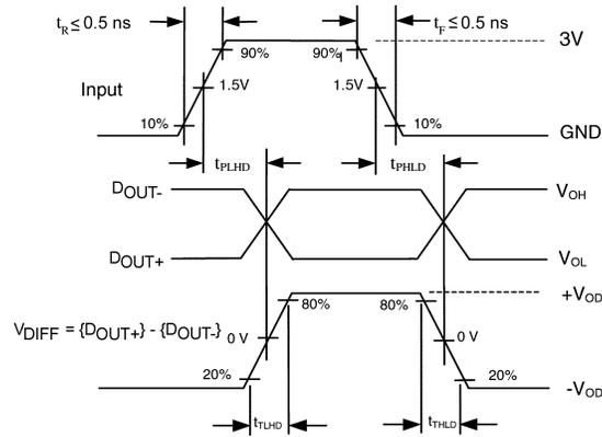
FIGURE 4. AC Waveforms
