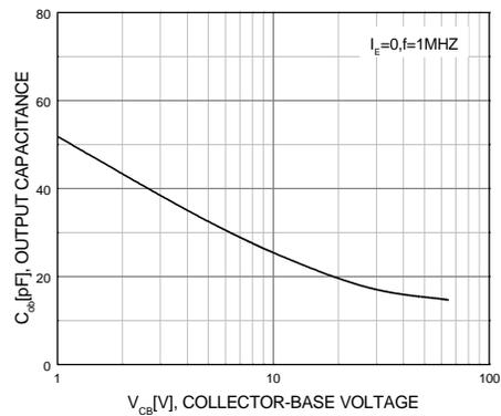
Figure 6. Collector Output Capacitance
