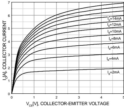
Figure 1. Static Characteristic
