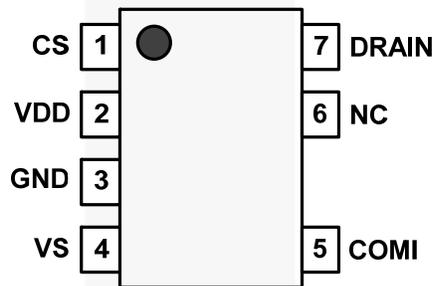
Figure 4. Pin Configuration
