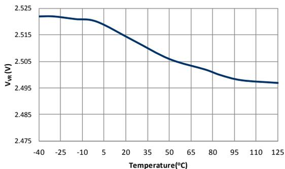
Figure 10. Reference Voltage ( $V_{VR}$ ) vs. Temperature
