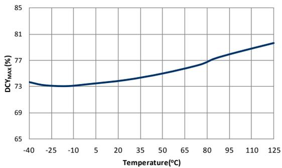
Figure 20. Maximum Duty Cycle ( $DCY_{MAX}$ ) vs. Temperature
