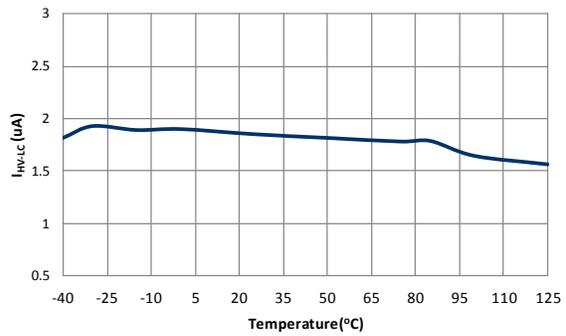
Figure 19. Leakage Current after Startup ( $I_{HV-LC}$ ) vs. Temperature
