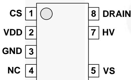
Figure 5. Pin Configuration
