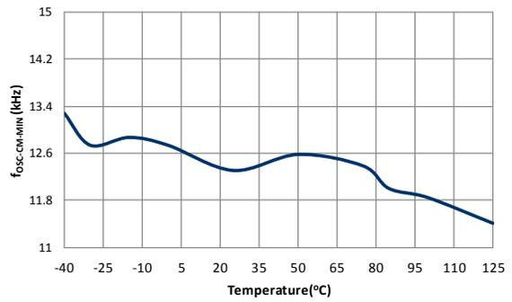
Figure 13. Minimum Frequency at CCM (f<sub>OSC-CM-MIN</sub>) vs. Temperature
