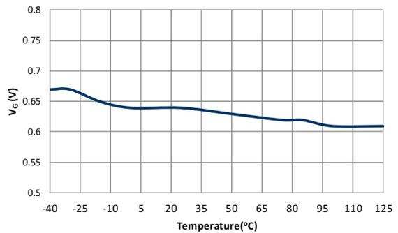
Figure 17. Green Mode Ending Voltage on EA\_V (V<sub>G</sub>) vs. Temperature
