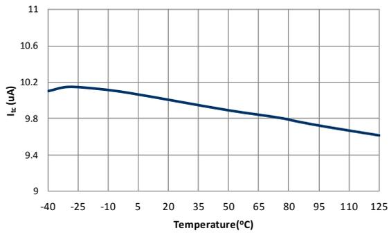
Figure 18. IC Bias Current ( $I_c$ ) vs. Temperature
