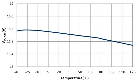
Figure 6. Turn-on Threshold Voltage ( $V_{DD-ON}$ ) vs. Temperature
