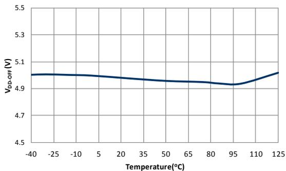
Figure 7. Turn-off Threshold Voltage ( $V_{DD-OFF}$ ) vs. Temperature
