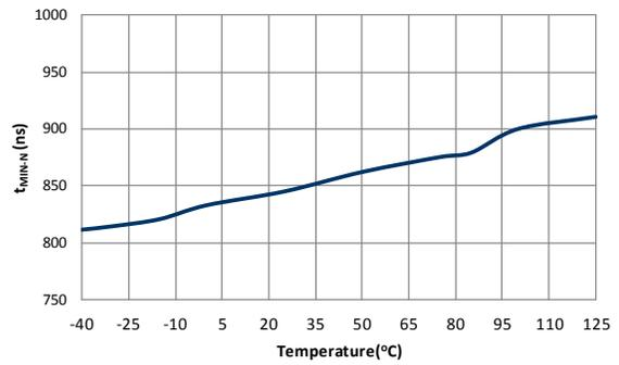
Figure 15. Minimum On Time at No Load (t<sub>MIN-N</sub>) vs. Temperature
