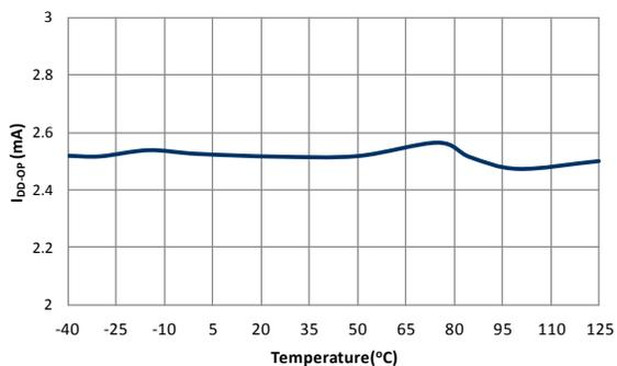
Figure 8. Operating Current ( $I_{DD-OP}$ ) vs. Temperature
