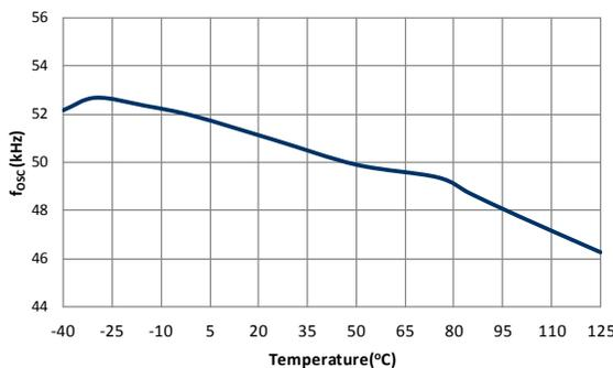
Figure 9. Normal Frequency 1 ( $f_{OSC}$ ) vs. Temperature
