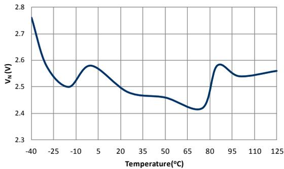
Figure 16. Green Mode Starting Voltage on EA\_V (V<sub>N</sub>) vs. Temperature
