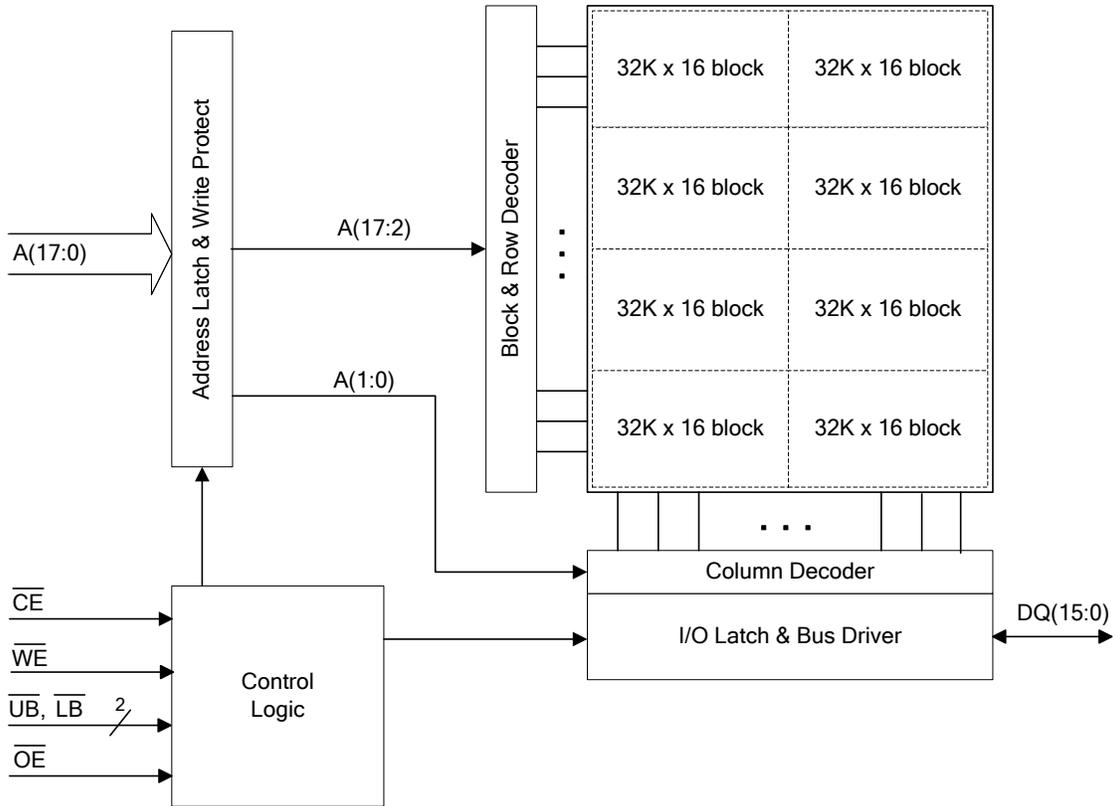
Figure 1. Block Diagram
