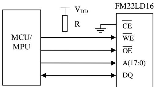
Figure 3. Use of Pullup Resistor on /WE
