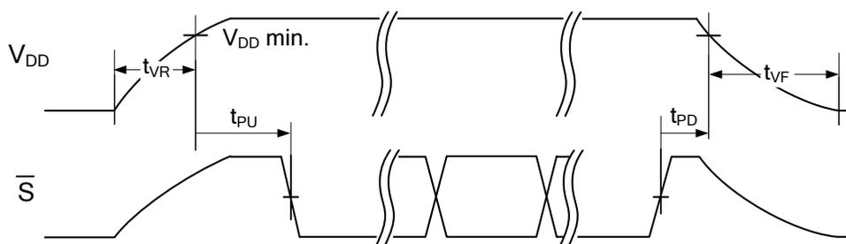
**Power Cycle & Sleep Timing** ( $T_A = -40^\circ\text{C}$  to  $+85^\circ\text{C}$ ,  $V_{DD} = 2.0\text{V}$  to  $3.6\text{V}$ , unless otherwise specified)
