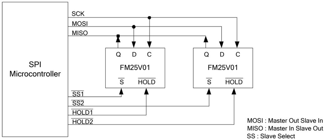
**Figure 3. 256Kbit (32KB) System Configuration with SPI port**
