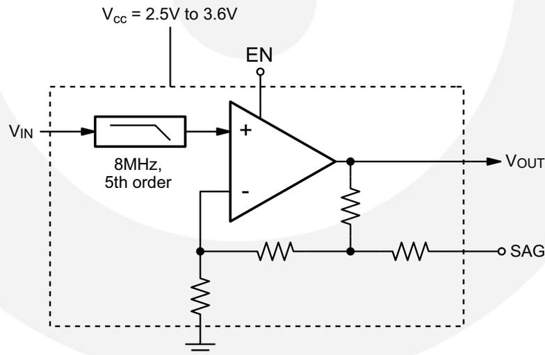
Figure 1. Block Diagram
