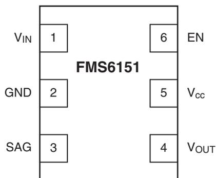
Figure 2. Pin Assignments
