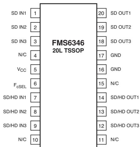
Figure 2. Pin Configuration
