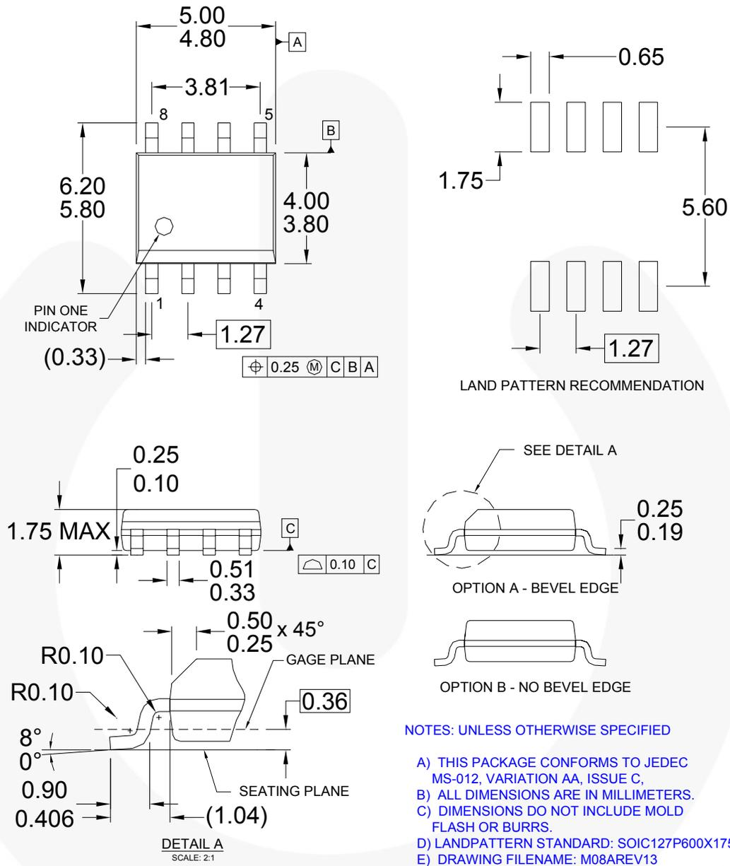
**Figure 5. 8-Lead Small Outline Integrated Circuit (SOIC) Package**
