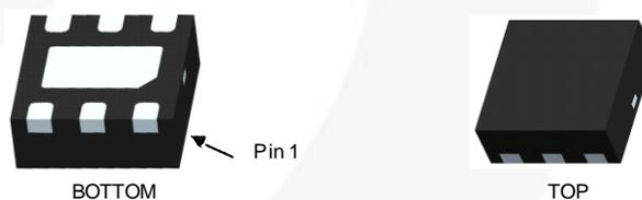
Figure 1. 2 mm x 2 mm Molded Leadless Package (MLP)
