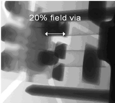
Figure 22: X-Ray result (bottom view with 45° angle)
