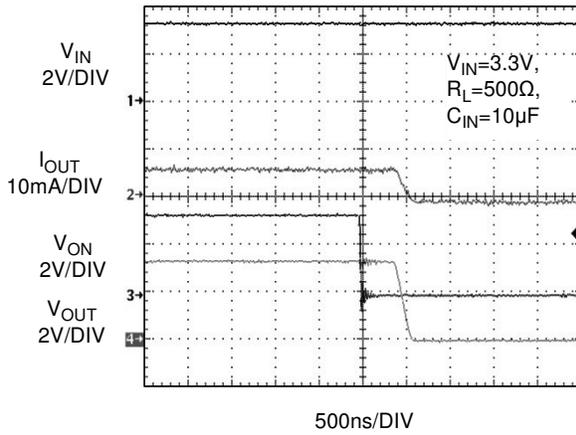
Figure 15.  $T_{OFF}$  Response
