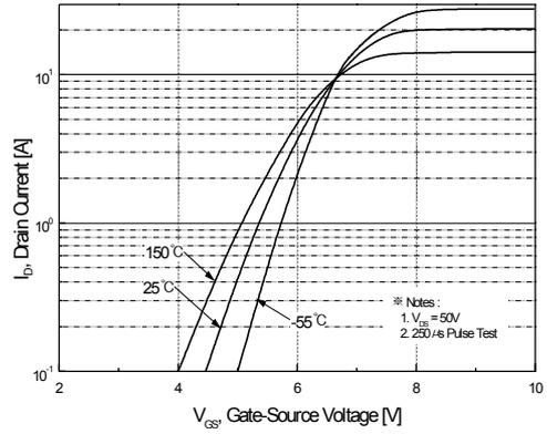
Figure 2. Transfer Characteristics
