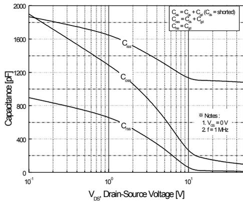
Figure 5. Capacitance Characteristics
